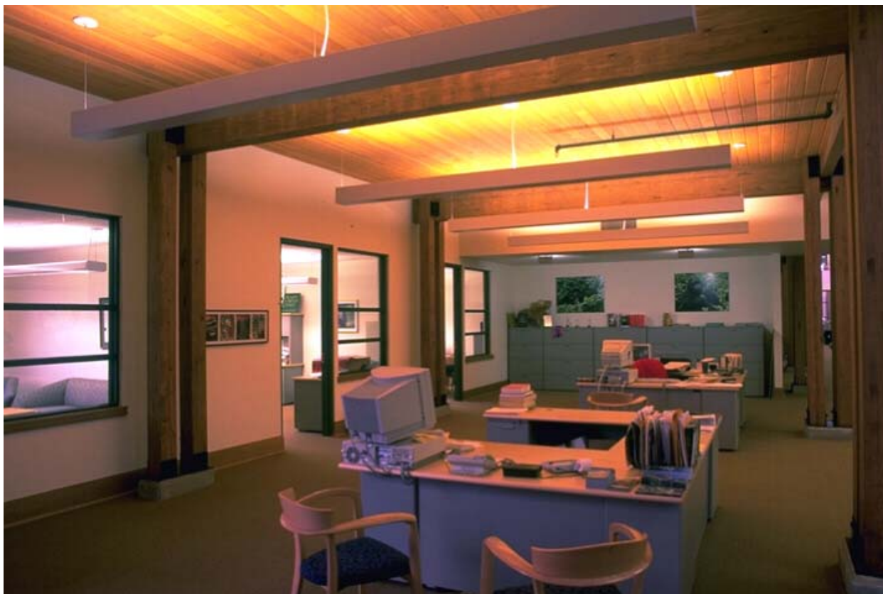
Figure 4 Minimize direct glare with indirect lighting.
