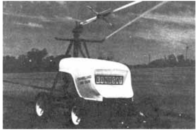
Figure 14-14. Traveling gun sludge sprayer (courtesy of Lindsay Manufacturing Company).
