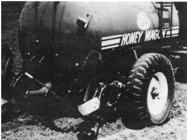
Figure 14-12b. Sweep shovel injectors with covering spoons mounted on tank wagon (Cunningham and Northouse, 1981).
