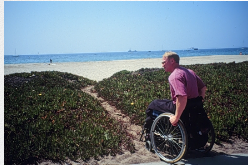
Figure 17-4. Unimproved paths, such as the one pictured here, typically connect the off-beach facilities, such as parking, playgrounds, or concession stands, to the edge of the beach. Beach paths with improved access should be designed at regular intervals along a beach.
