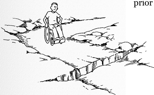
Figure 15-7. This sudden change in the natural ground level is a potential safety hazard for hikers and other trail users.
