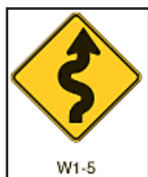
Winding Road sign for three or more alignment changes in close proximity.
