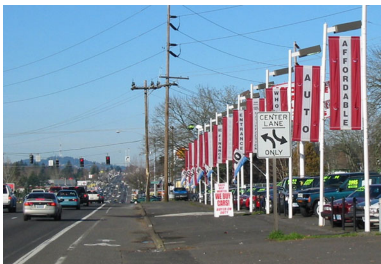
Figure 2. In terms of both official signs and advertising displays, too many displays may have the effect of causing drivers to “tune out,” and recall will be poor. This photo shows an example of sign clutter where the regulatory sign is difficult to isolate from the background advertising signs.
