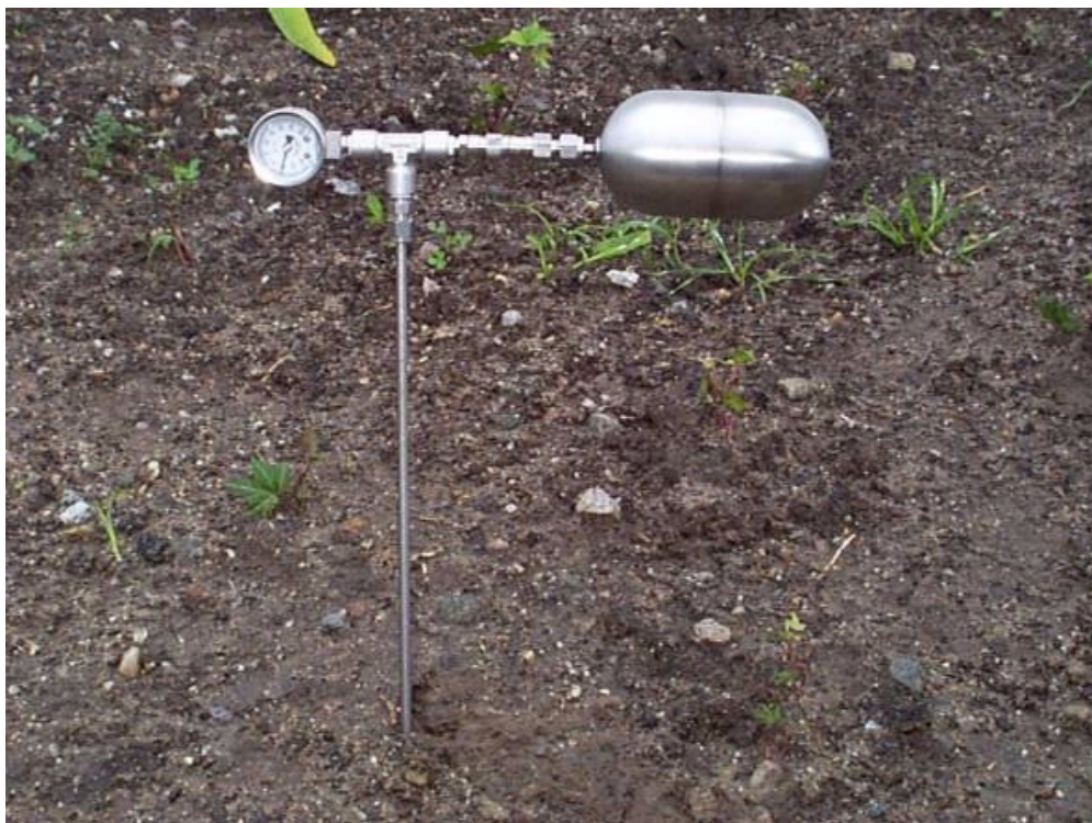
Figure A-9. Application of EPA's Compendium Method TO-15 for VOCs at a MSW Landfill.
