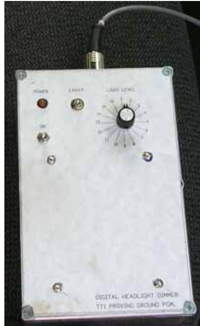
Figure 14. Photo. Headlamp controller box.
