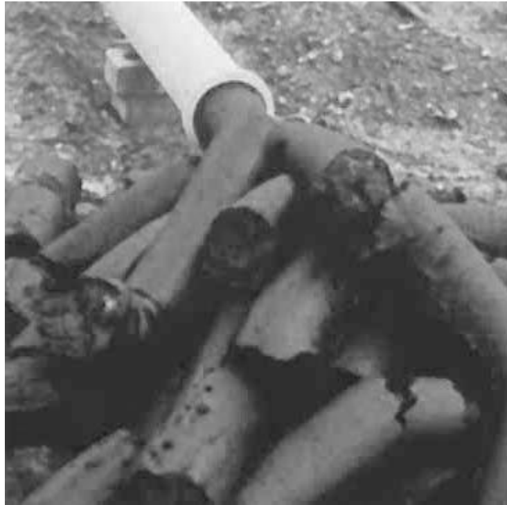
Figure 7. Extruded High Solids Sludge from Piston Pump (Courtesy of Schwing Bioset, Inc.)
