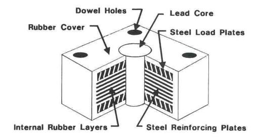
Figure 9.1.15 Lead Core Isolation Bearing
