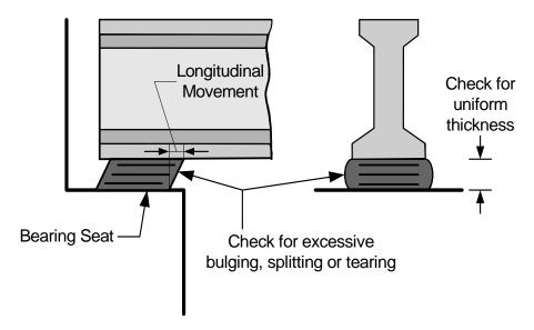
Figure 9.1.34 Elastomeric Bearing Inspection Checklist Items
