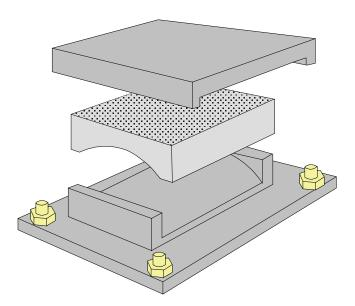
**Figure 9.1.6** Self-lubricating Bronze Sliding Plate Bearing
