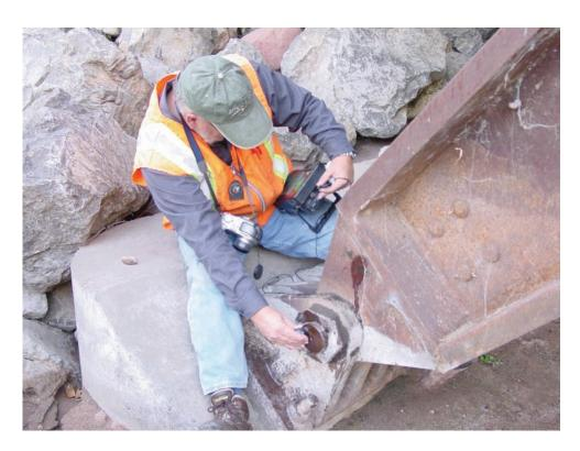
Figure 9.1.21 UT Inspection of a Pin in a Bearing
