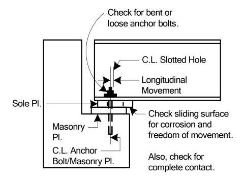
Figure 9.1.27 Sliding Plate Bearing Inspection Checklist Items
