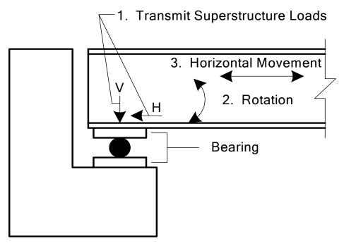
**Figure 9.1.1** Three Functions of a Bearing
