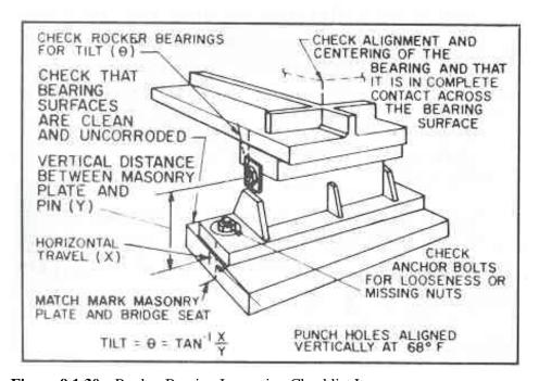
Figure 9.1.30 Rocker Bearing Inspection Checklist Items
