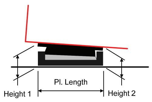
Figure 9.1.33 Angle of Rotation for Pot Bearing
