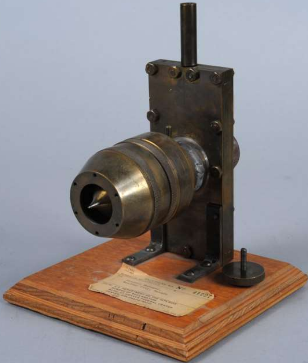
Left: needle valve model Above: body points for 84- inch balanced needle valves (on flat car in storage yard near Hoover Dam; May 1935)
