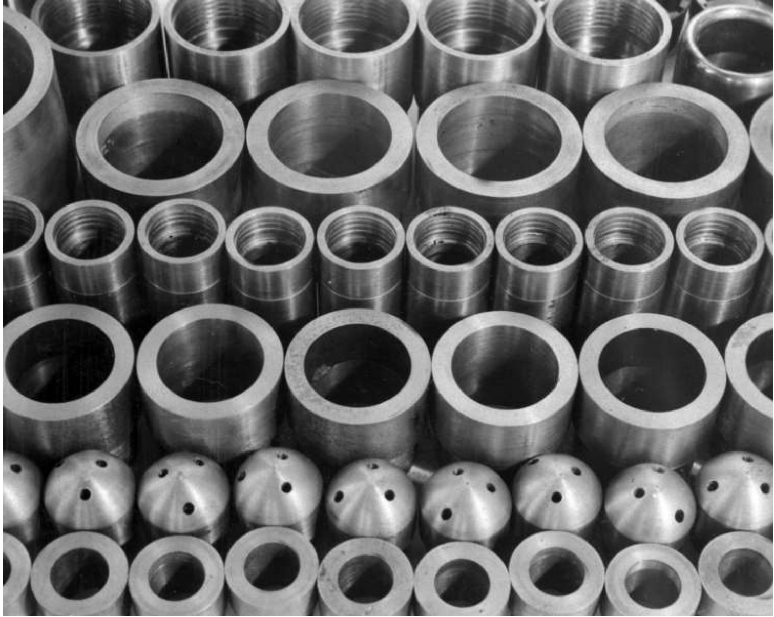
A pattern of new diamond drill core and plug bits (before diamonds have been set)
