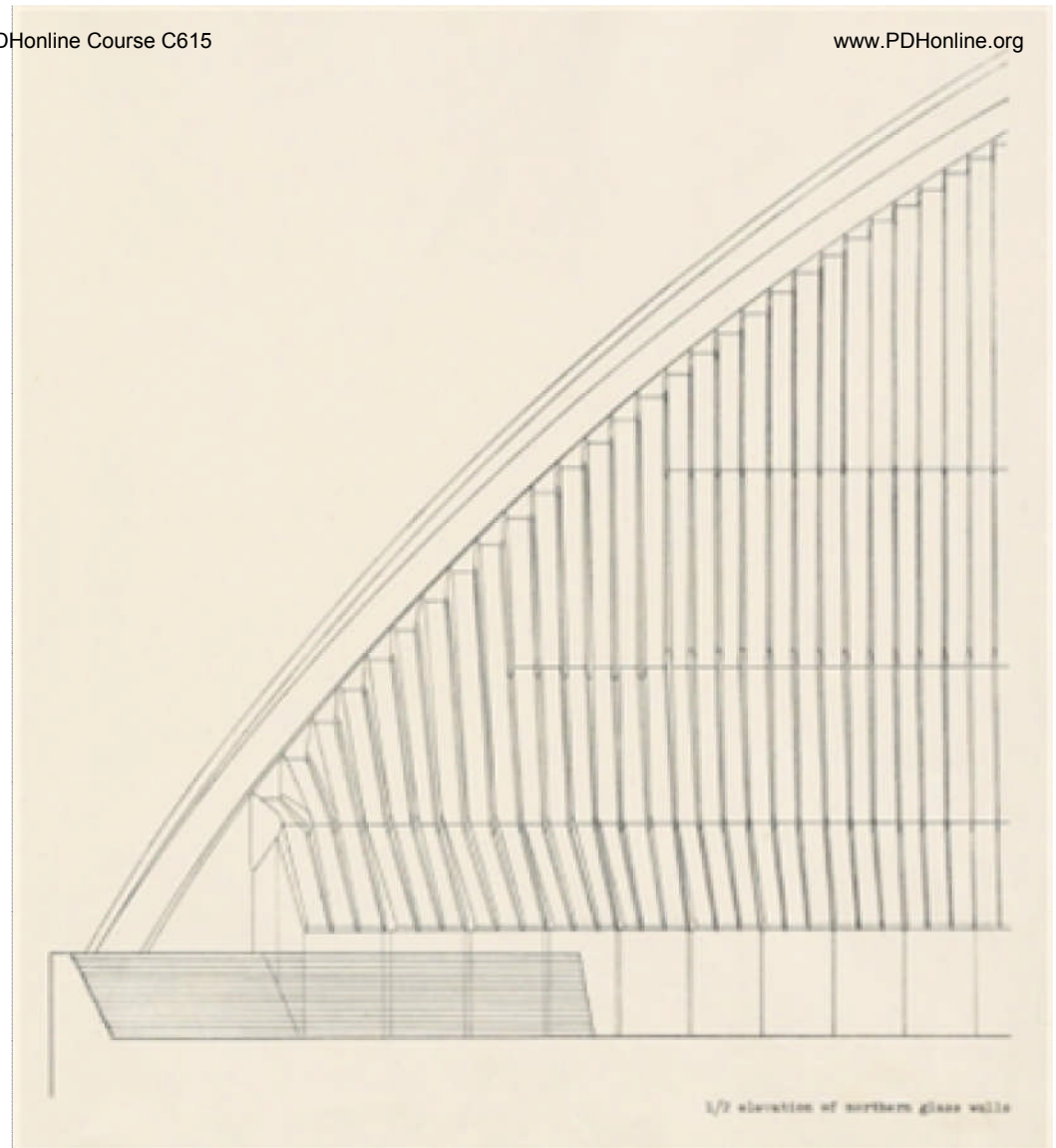
Section (left) and front elevation (right) of the northern glass walls (from the Yellow Book , 1962)
