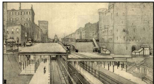
Above: caption: "A Three-Deck Street-Railway Crossroads. Three layers of street-railways are shuffled together at Fourth Avenue and Thirty-Fourth Street, New York. The picture, looking uptown, cuts away the street-paving at Thirty-third Street, exposing the Subway underneath. It shows on top (crossing the picture) a car of the Thirty-fourth Street crosstown line; in the middle, a car of the Fourth Avenue surface line, the tracks of which disappear into the tunnel at the steep Thirty-fourth Street hill; underneath all, the Subway. A downtown express is passing; the express tracks (in the middle) are sunken here, since expresses do not stop at Thirty-third Street. A downtown local is pulling up at the platform." 84 McClure's Magazine, March 1905
