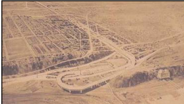
Above: caption: "Ultimate Arrangement of New Jersey Approach. Weehawken toll plaza with its connections to Hudson County Boulevard East and Park Avenue, the viaduct loop structure, and the open-cut express highway through Union City. The latter will provide connection with Hudson County Boulevard and state highway routes in North Bergen. The toll plaza is practically complete, while the viaduct structure and depressed highway 109 are now under construction." (as of December 1937)
