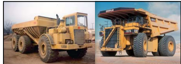
Left: caption: "Articulated dump truck: DJB D350. The articulated dump truck resembles a prime mover and rock wagon, but it's built as a complete unit and all wheels are powered. The largest carries 55 tons." Right: caption: "End dump truck: c. 1997 Cat 797B. End dumps used in mining are quite large. The Cat 797B, for example, had a working weight of 687.5 tons and was rated at 3,550 horsepower and 380 tons capacity."
