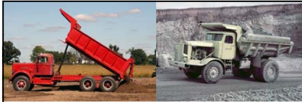
Left: caption: "Dump truck: 1961 White Super Mustang. Heavier loads require more tires on the ground to carry it. This tandem-axle truck carries up to ten cubic yards." Right: caption: "End dump truck: Euclid 46TD. Purpose-built off-highway end dumps were invented in 1935. This 1950s model carried 22 tons; trucks for construction and quarrying are usually rated under 100 tons."
