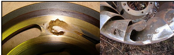
"...The hammering of the water as the bubbles collapse creates vibrations, limits speeds and actually corrodes metal. Fast ocean liners must sometimes go into dry dock for repairs to propellers that have been eaten away by cavitation. Engineers know what causes cavitation and they know its harmful effects but they don't know for certain how it works..." Popular Mechanics, July 1949 Left: caption: "Cavitation damage on a valve plate for an axial piston hydraulic pump" Right: caption: "Cavitation damage to a Francis turbine" 123
