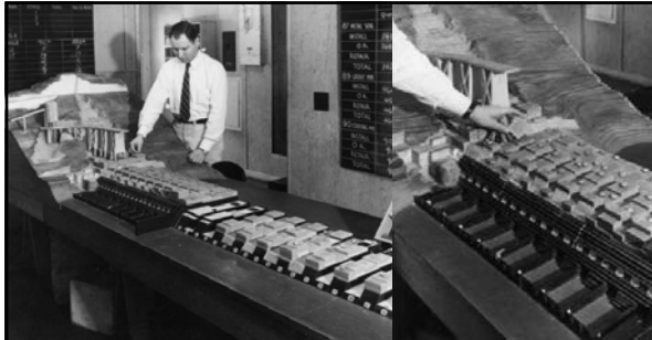
"...the model will be fitted so that the excavation areas can be lifted out, displaying the present finished slopes. The cofferdam can then be put in, as well as the cross-stream coffer, to show the methods of diversion. A wooden model of the dam will be built, which can be slipped in place, to show how the completed project will look. The finished model will weigh about 400 pounds..." Spokesman-Review, April 24 th 1936
