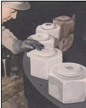
Popular Mechanics, May 1942 Left: caption: "These huge nuts, used to couple the shaft of the waterwheel to the generator rotor, were shrunk with Dry Ice to 80 degrees below zero so they will expand and tighten after fitting" 1577
