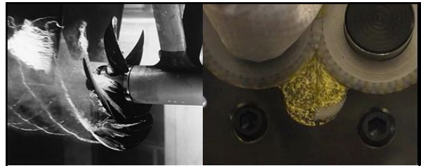
"When an object moves under water at high speed a mysterious force is brought into play that has baffled scientists for years...The mysterious force which acts as a brake on any speeding underwater object is known as cavitation. This bugaboo of hydrodynamics is something like the drag that limits the efficiency of airfoils in the atmosphere. A swiftly moving body creates a cavity in the water in the form of a blanket of low-pressure bubbles that appear, grow and collapse..." Popular Mechanics, July 1949 Left: caption: "Cavitating propeller model in a water tunnel experiment" Right: caption: "Cavitation in a gear pump" 122
