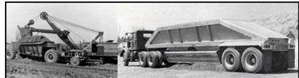
Left: caption: "Bottom dump truck: c. 1941 Euclid FDT. Invented in 1935, the off-highway bottom dump truck was much larger and faster than horse-drawn or crawler wagons. Capacity ran from 13 to 100+ cubic yards." Right: caption: "Bottom dump trailer: After World War II, the bottom dump concept was adapted for use over the road behind truck tractors. Typical capacity was 12 to 24 cubic yards."
