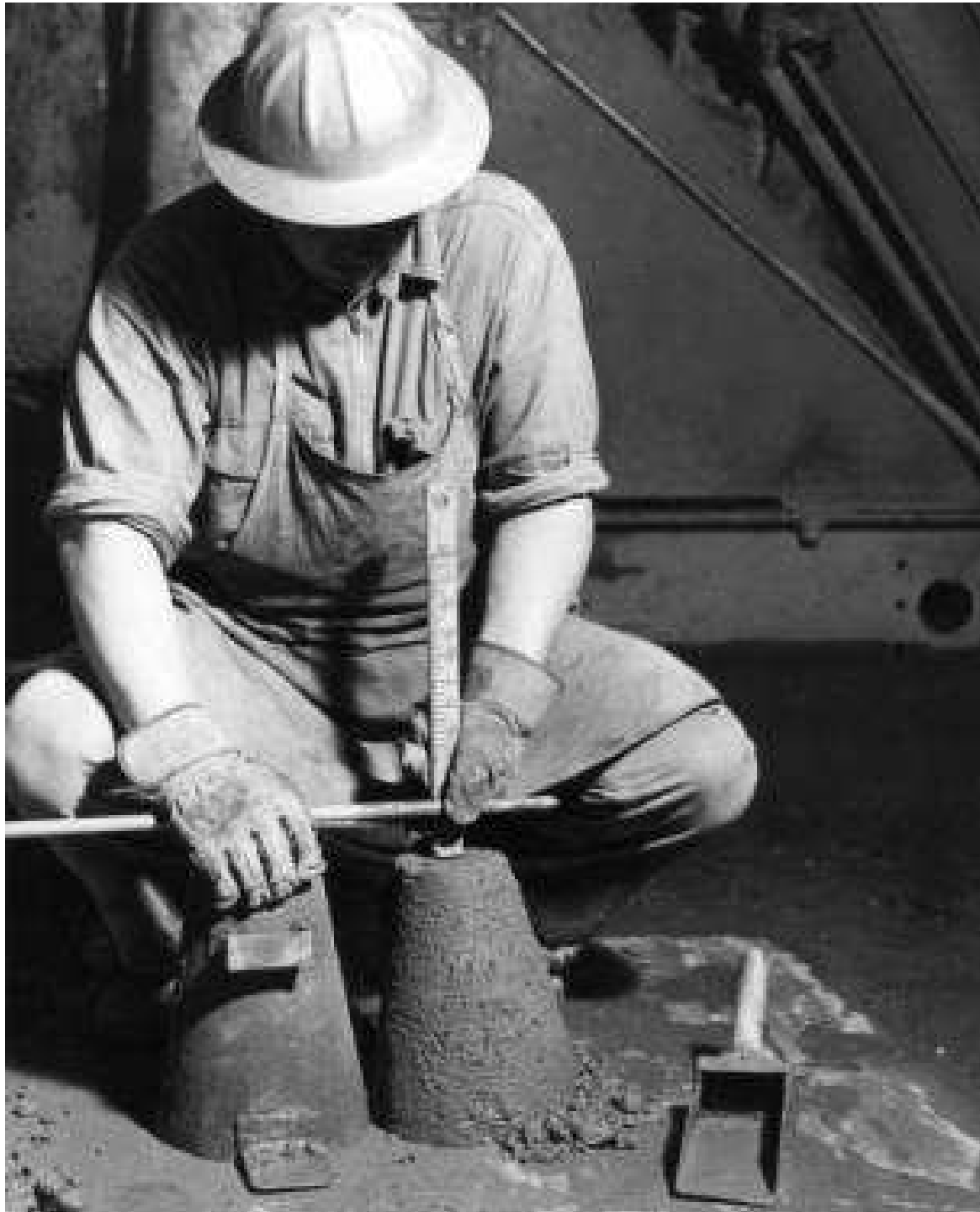
Above & Left: caption: “Gov’t. inspector filling cyl- inder with concrete sample at plant for slump test, June 1940”
