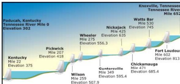
**Above:** caption: "Nine main-river dams form a 'staircase' of quiet, pooled water and controlled current - a continuous series of reservoirs that stretches along the entire length of the Tennessee River. From its beginning just above Knoxville, the Tennessee drops a total of 513-feet in elevation before it joins the Ohio River."
