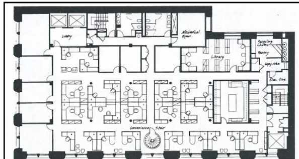
Above: caption: "Drawing of a typical floor plan at Audubon House. The central workspaces feature open plans with modular workstations, enhancing the daylighting of the interior. Enclosed offices are grouped along the western and northern perimeters, minimizing interference with daylighting, and core elements (elevators, fire stairs, pantries, and mechanical rooms) are grouped on the north and east solid exterior walls, away from the sunlit southern and western exposures." 126
