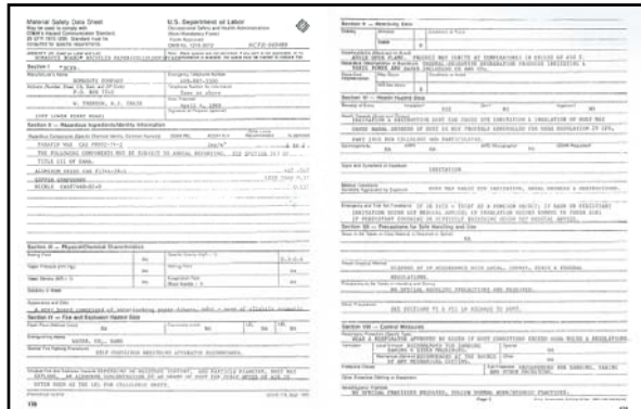
Above L&R: caption: "Every manufacturer of a building material is required by law to provide a MSDS sheet (sample above). Following standards set by OSHA, the sheet lists percentages and names of hazardous materials that are components of a product. However, trace amounts of chemicals/toxins are not required to be listed." 157
