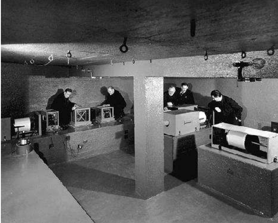
Above L&R: caption: “Vertical, North-South, and East-West Galitzin-Wilip Seismometers at the Florissant, MO vault. Recording drum pictured in bottom photo, left of seismometers.”
