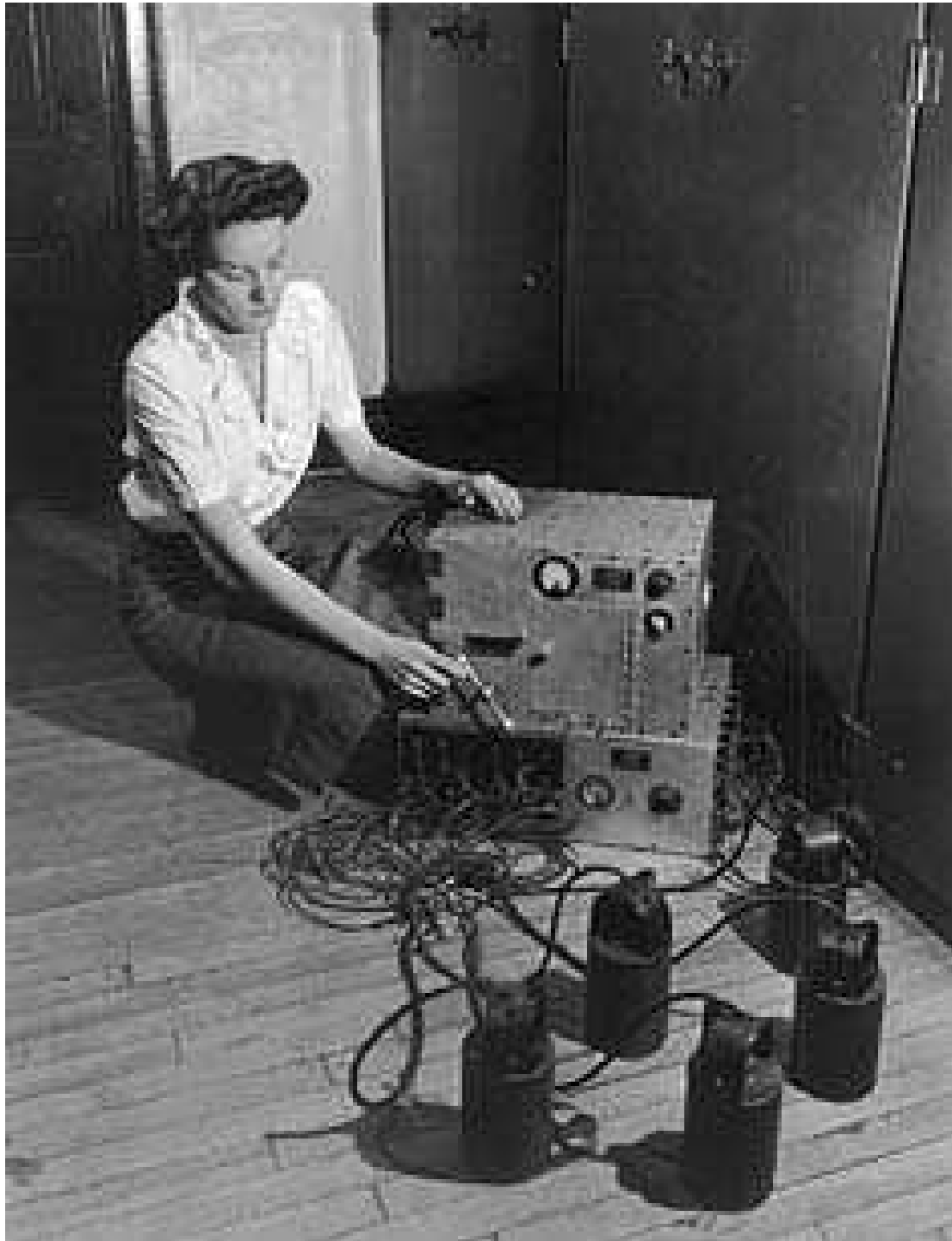
Above: caption: "Seismograph Service Corporation Type Reflection Seismometers, Amplifiers, and Camera"
