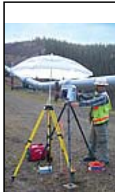
Left: caption: "CMSI-Bell surveyor Greg Johnson shields the Trimble 3D scanner from rain in order to survey TAPS at Lost Creek Hill, approximately 80 miles NE of Fairbanks, Alaska"
