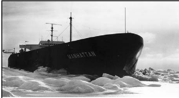
"...Now, out in Viscount Melville Sound, the ship was behaving perfectly, battering through nine-foot-thick ice at a steady six knots (normal cruising speed is 16.5 knots). An ordinary icebreaker rises and falls with a rolling motion as it slides up on the ice and crashes down through it. But the Manhattan is so massive that it plows straight ahead..." Popular Science, January 1970 229
