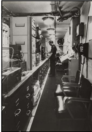
Left: caption: "A technician checks some of the navigational equipment that will guide the SS Manhattan on its Northwest Passage voyage. Among the vast array of sophisticated equipment used in navigation will be special-purpose earth satellites placed in polar orbit under the U.S. Navy Navigation Satellite System program. Impulses from these satellites linked with those from sonar, accelerometer and gyro signals comprise the integrated system that will guide the ship." 241
