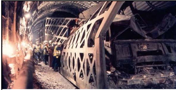
In 1996, 2006 and 2008, trains carrying both vehicles and passengers caught fire. The original plan was to keep moving in the event of a fire; passengers would move into the undamaged part of the train, which could then be detached and driven out of the tunnel safely. After the 1996 fire (above) this policy was changed to evacuate passengers as quickly as possible, moving them into the service tunnel which runs between the two train tunnels. 1627
