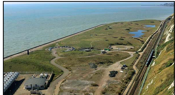
Above: caption: "Once construction works for the Channel Tunnel were completed, the site was landscaped to provide an undulating topography including some low-lying wetlands. The Samphire Hoe country park opened on 17 July 1997. This view from Shakespeare Cliff dates from March 2014. The building on the left is part of the ventilation system for the Channel Tunnel. Air is supplied to the Channel Tunnel from here and a similar plant at Sangatte. Either of the two buildings is capable of supplying all the air required to ventilate the tunnel. Supplementary ventilation also exists on either side of the tunnel. In the event of a fire, ventilation is used to keep smoke out of the service tunnel and move smoke in one direction in the main tunnel to give passengers clean air."
