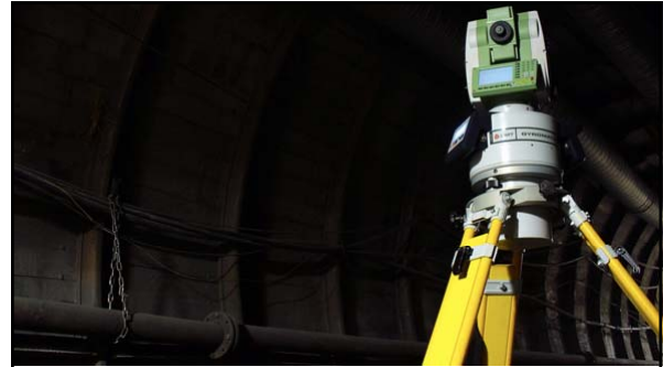
Underground, a compass doesn't work due to magnetic ore and GPS can't function. Fortunately, in 1921, Max Schuler invented a gyrotheodolite (above) which uses the rotation of the Earth to calculate direction. However, due to problems on the French side of the tunnel, Fagg and Cozette didn't actually meet in the center of the tunnel. With the Brits digging a little further, when the two tunnels did meet, they were 300-millimeters off course.
