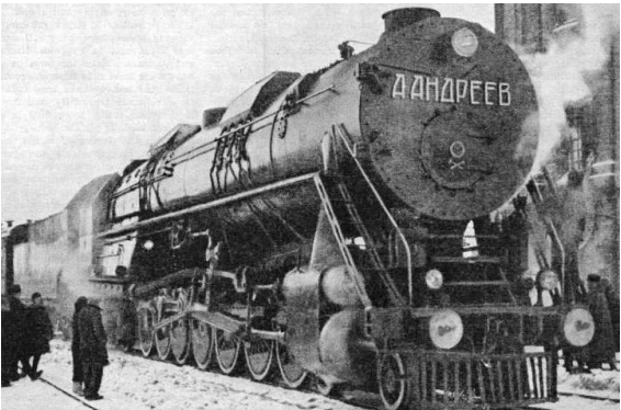
Caption: “EUROPE’S MOST POWERFUL GOODS ENGINE. This is the claim made for the large freight engine, seen here on its arrival in Moscow in January, 1935. It was designed for hauling coal trains of 3,000 tons from the Donetz mines to Moscow.”
