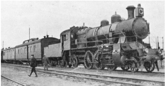
Caption: “A TRACK GAUGE OF 5-FEET and a generous constructional or loading gauge make possible the building of exceptionally tall locomotives in Russia. A Russian engine may be built to a height of 17-feet from rail-level to chimney top. The 2-6-2 locomotive at the head of the train illustrated has a peculiarly Russian characteristic. This is a railed-in gallery extending from either side of the cab round the smokebox. The 5-foot track gauge is peculiar to Russia and to some bordering countries formerly Russian. Through running from other countries is therefore impossible, but within the Soviet Union enormously long through train journeys are possible.”
