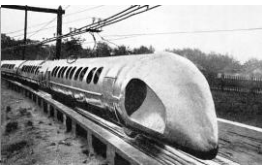
Above: caption: “FUTURE DEVELOPMENTS are foreshadowed by this electric train which runs along on balls instead of wheels. This novel device was the idea of a young Soviet inventor. Experiments are reported to have given satisfactory results. The picture shows the experimental track.”
