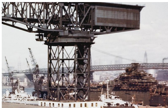
901 Caption: "The U.S. Navy aircraft carrier USS Franklin (CV-13) under repair New York Naval Shipyard on 27 October 1945. The entire flight deck and supporting upper hull was removed and rebuilt because of the extensive damage caused by two Japanese bombs that penetrated the flight deck on 19 March 1945, 901 exploding on the hangar deck, igniting fuel and ordnance from the aircraft below decks."
