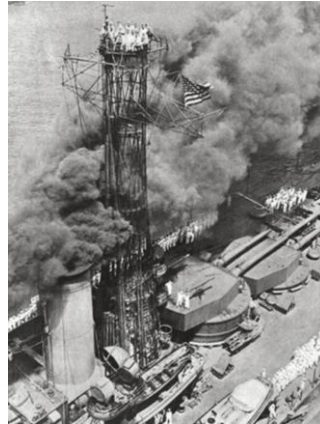
Oil-soaked coal used to fire the boilers (in an age when Navies were converting over to oil, which was a much more efficient fuel) produced vast clouds of smoke pouring from her funnels. However, the propulsion system followed the modern trend of steam turbines (paradoxically, the USN went back to reciprocating engines on its next class of battleships). During WWI, the Wyoming served dutifully on patrols. In 1931, the ship was converted into a gunnery training ship, with all of the gun mounts proving very useful in providing platforms to train naval gunners. Caption: "Bird's-eye view of the deck of the U.S.S. Wyoming, showing the fighting mast crowded with sailors and the two turrets amidships, photographed from a tower of the Manhattan Bridge, New York City." 668
