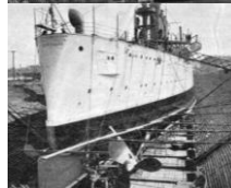
Upper Left: caption: "New armored cruiser 'Colorado' in dry dock at the Brooklyn Navy Yard. Her successful trial trip over the Cape Ann course, in which the vessel averaged 22.24 knots-an-hour, marks this vessel as the fastest armored warship in the Navy. Previously, the armored cruiser 'Brooklyn' was the fastest vessel carrying side armor "
