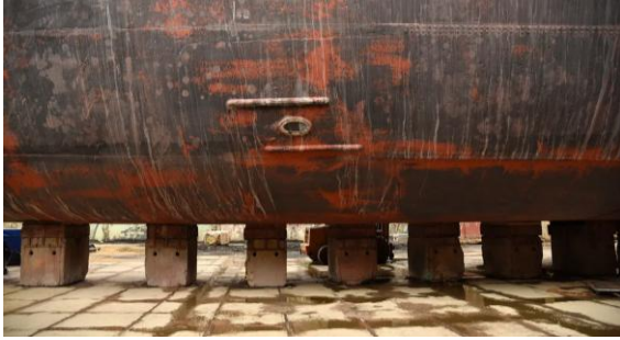
“...Although it seems precarious, the entire weight of this 12,892-ton vessel is supported by a carefully arranged set of dry dock blocks. ‘Our barges are a little bit easier to dock, because they are square and flat,’ explains Sanborn. ‘Our Coast Guard vessels and our ships are a little bit more difficult’...” ny.curbed.com, May 3, 2018
