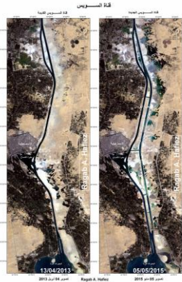
“...Suez is simpler, lock-free, and large enough to handle oversized ships, but only if they transit in convoys, with bypasses allowing the convoys to pass one another. To allow more room, workers are digging a new canal parallel to 22 miles of the existing one and expanding the current bypasses. The result will be a new 45-mile lane, expected to open this fall, that should reduce ships’ journeys by at least 12 hours...” popularmechanics.com, August 18, 2015 Caption: “Old vs. new Suez Canal”
