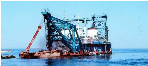
Caption: "The first modern initiatives to improve the Suez Canal occurred in the 1950s. These improvements were followed by the largest widening and deepening works from 1975 to 1980 when a huge dredging fleet of 12 cutter suction dredgers dug-out 225 million m³ for the 63 kilometers between Lake Timsah and the Great Bitter Lake. The third intervention occurred from 1992 to 1994 when, as part of a plan to handle fully loaded tankers, the canal was widened by 45-meters and the channel deepened to -25 meters. During this phase, some 17 million m³ of bedrock material – 5x harder than normal concrete – were dredged." 257
