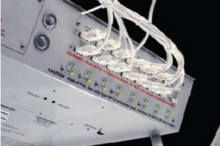
16-channel power module with Class 2 output circuits
