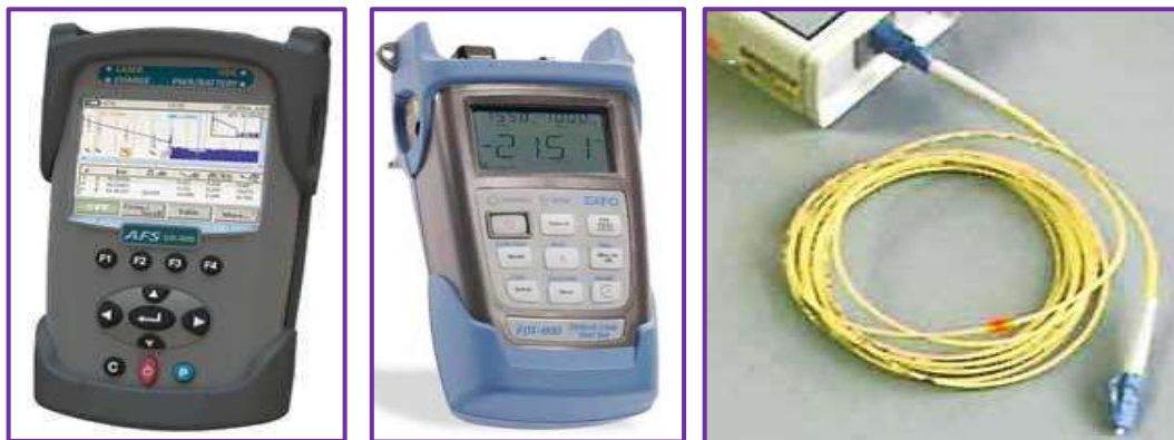
Optical Time Domain Reflectometer; OLTS (Optical Loss Test Set); Visual Cable Tracers and Fault Locators
