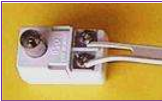
A 75-to-300 \Omega balun built into the antenna plug. Three audio transformers, two of them baluns.
