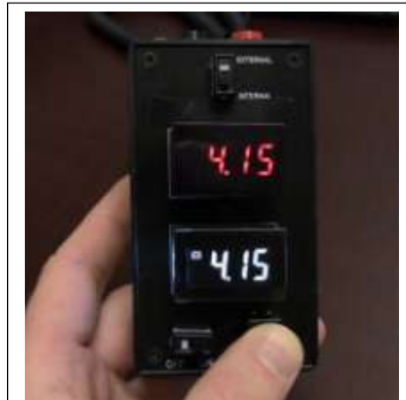
Fig. 2 - Panel Mounted Meters
