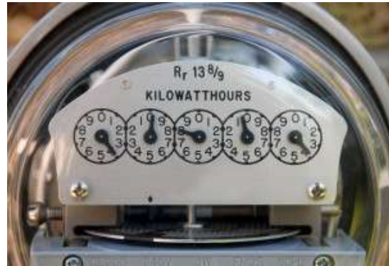
Fig. 6 - Conventional Watt-hour Meter
