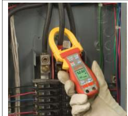
Fig. 3 – Clamp-on Single Phase Power Meter
