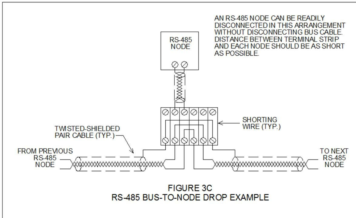
RS-485 networks often are used in applications like building HVAC (Heating, Ventilation and Air Conditioning) systems, where system parameters change slowly and fast communication is not essential.
