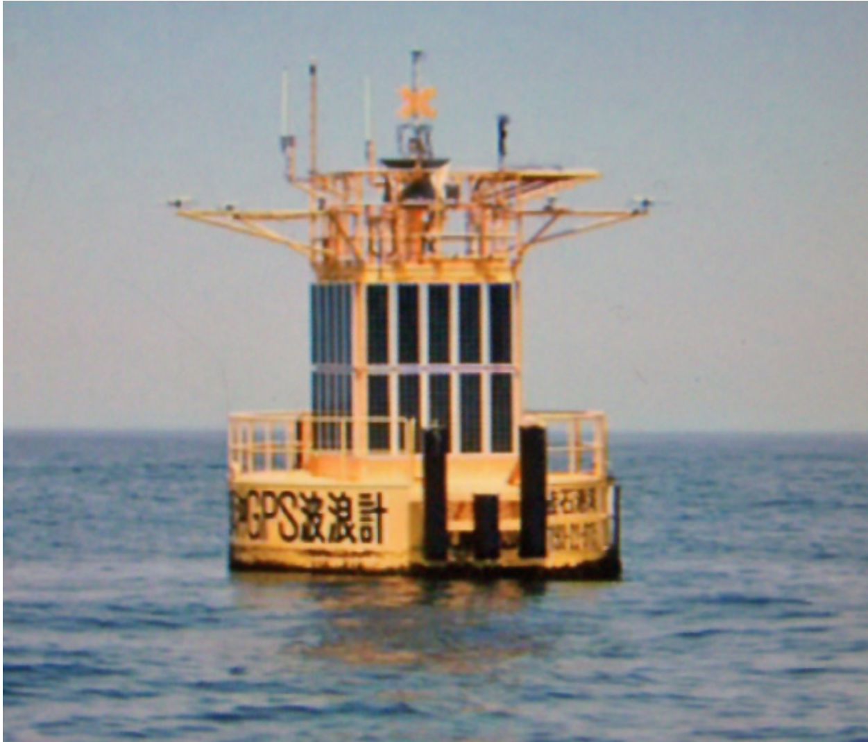
Figure 15: Type of GPS buoy deployed in the ocean off the Eastern Coast of Japan to record real time changes in sea level.
