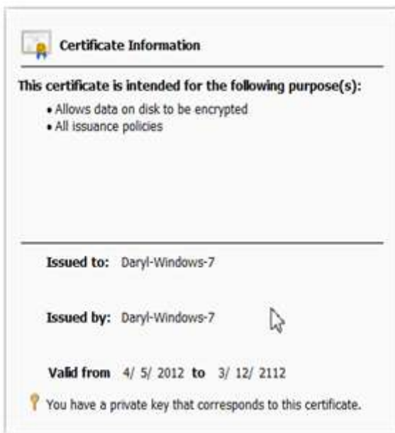
Figure 5 shows the Issuer to and by fields are the same for Self-Signed Certificates.
