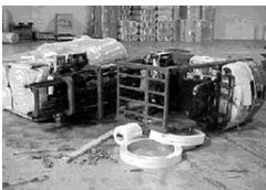
Overturned forklift resulted in fatality.
