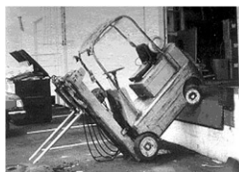
Forklift driven off loading dock.
