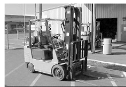
Safety features include an overhead guard.
