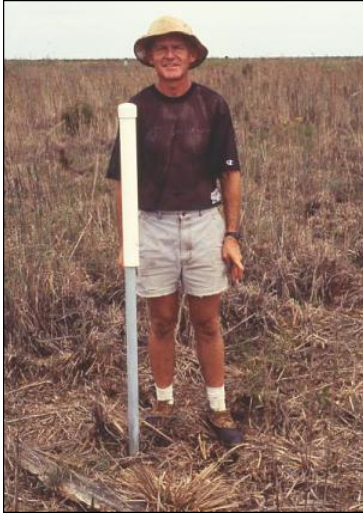
Figure 12. Stainless steel piezometer, courtesy of Fish & Wildlife Service.
