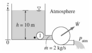
In the absence of any changes in flow velocity and elevation, the power produced by an ideal hydraulic turbine is proportional to the pressure drop of water across the turbine.
