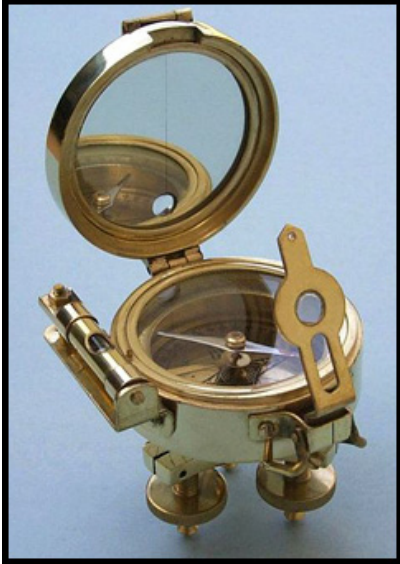
Contemporary reproduction of an early surveyor's compass.
