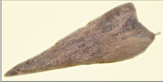
Figure 15. Old cedar hub excavated at a property corner. Note the nail set during a recent survey.
