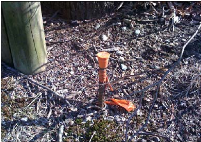
Figure 20. 3/4" iron rebar with plastic identification cap.
