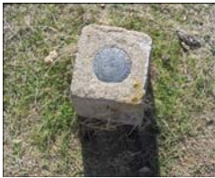
Figure 41. USGS horizontal control point.
