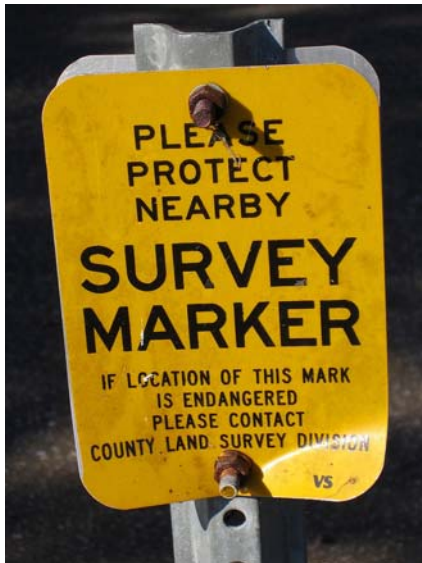
Figure 40. A county monument witness sign, Florida.
