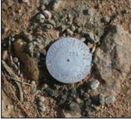
Figure 11. Aluminum alloy corner, City of Los Angeles.
