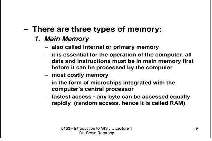
The main memory is the memory which is referred to as RAM. Random Access Memory (RAM) provides space for your computer to read and write data accessed by the CPU. RAM is relatively, very expensive memory because it is the memory which is required to run the application programs, operating system, and the data sets for the programs.
