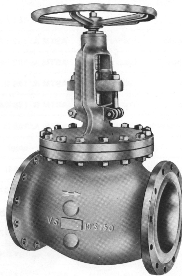
Figure 3-9. Globe Valve, Standard Pattern, Bolted Bonnet, External Screw, Plug Disc. (Courtesy of Crane Co.)
