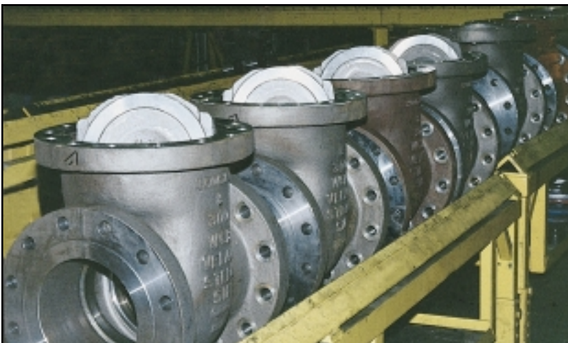
7 Assigning the ideally fitted wedge, ground and lapped, to proper valve body.
