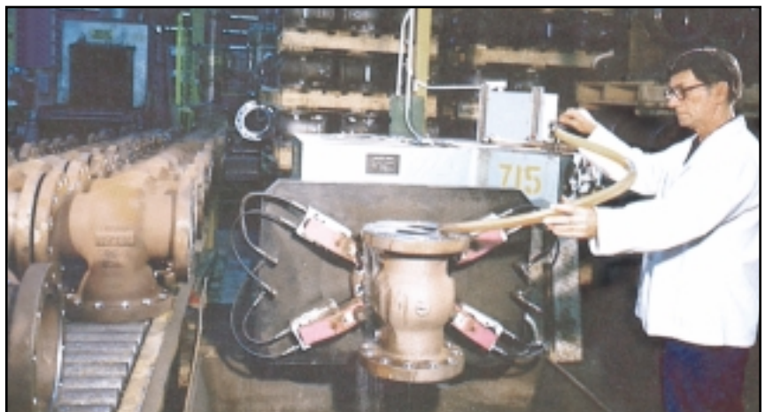
2 Air-under-water test of the seat's welds.
