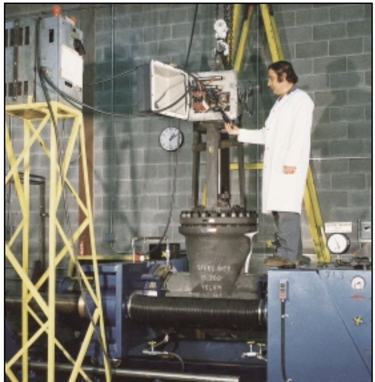
All valves are tested during production for reliability with pressurized air and hydrotested for bubble-free tightness in accordance with API 598 specifications.
