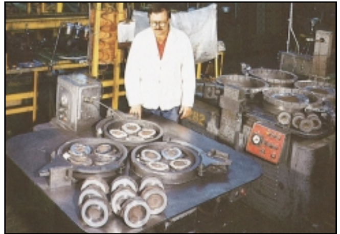
6 Lapping of wedge seating surfaces.
