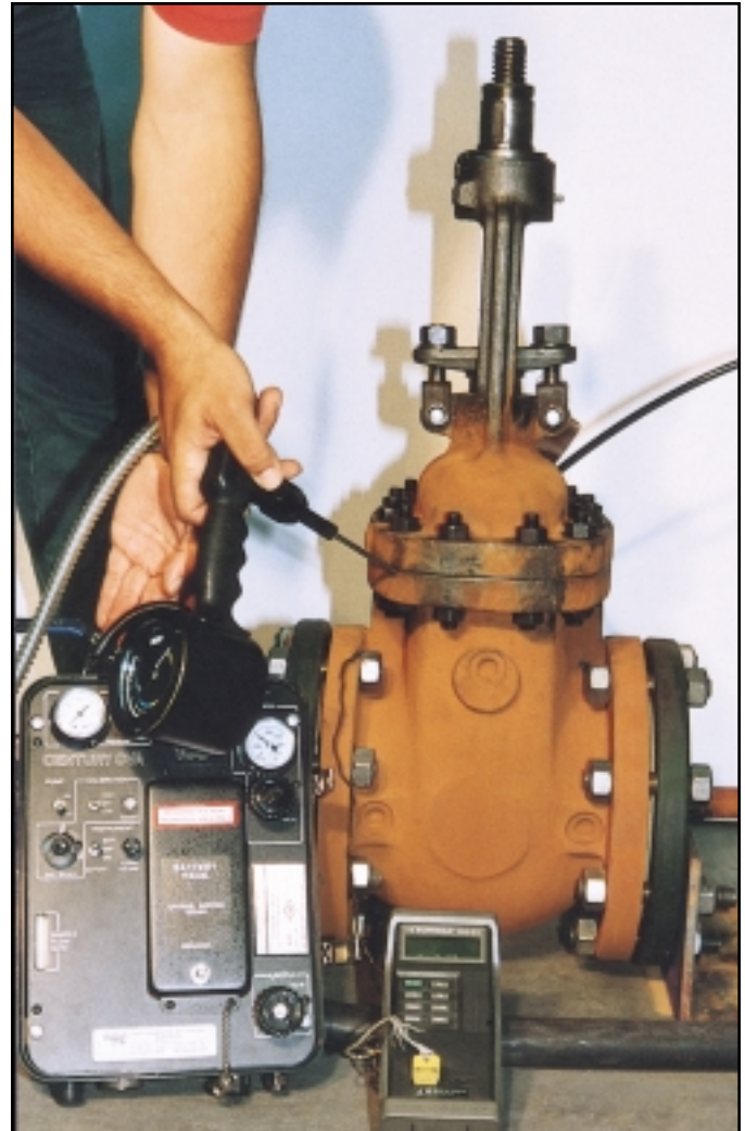
Upper right: 50 cycles with steam at 400°F (204°C) Leakage: zero ppm.
