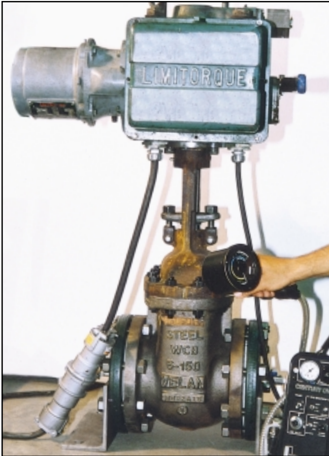
Upper left: 3000 cycles with propane at 125 psi Leakage: zero ppm.
