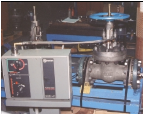
All valves are tested during production for reliability with pressurized air and hydrotested for bubble-free tightness in accordance with API 598 specifications.
