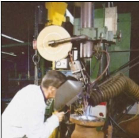
1 Automatic seal welding of Stellite 6 hardfaced seats.
