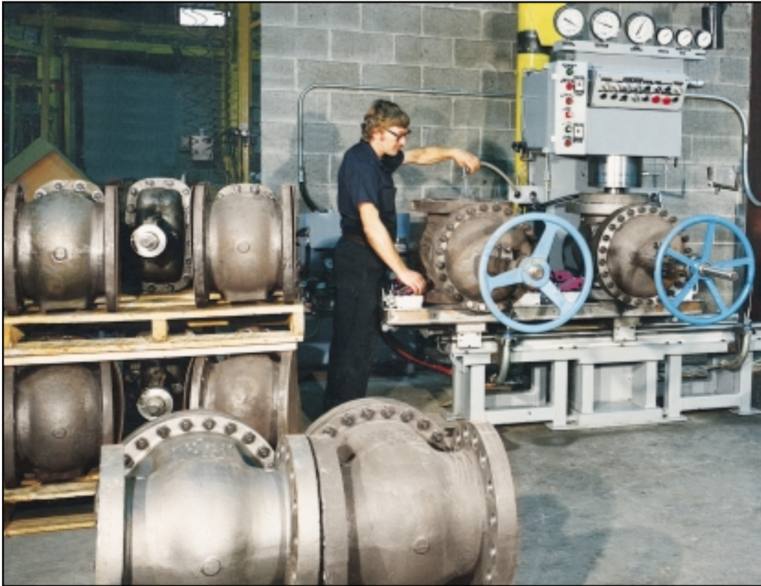
Top: Semi-automatic stations for testing 2–12" (50–300 mm) valves to API 598.
