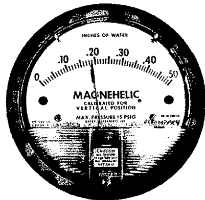
Figure A-44. Magnehelic Gauge. Courtesy Dwyer Instruments, Inc.
