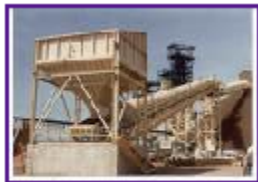
54" wide belt conveyor with ship unloading hopper feeding a traveling tripper conveyor for storage
