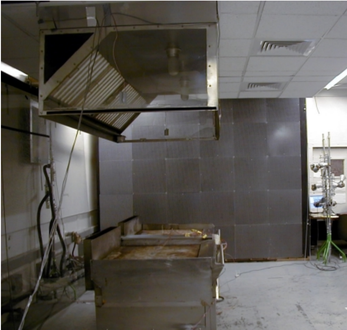
Figure 55: Test Set-Up for Exhaust Only Canopy Hood and Two Gas Griddles as Viewed from the Schlieren Optical System
