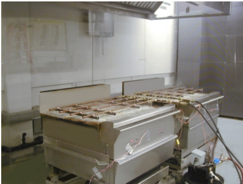
Figure 14: Two Gas Griddles under a Canopy Hood with the Cooking Simulator Installed
