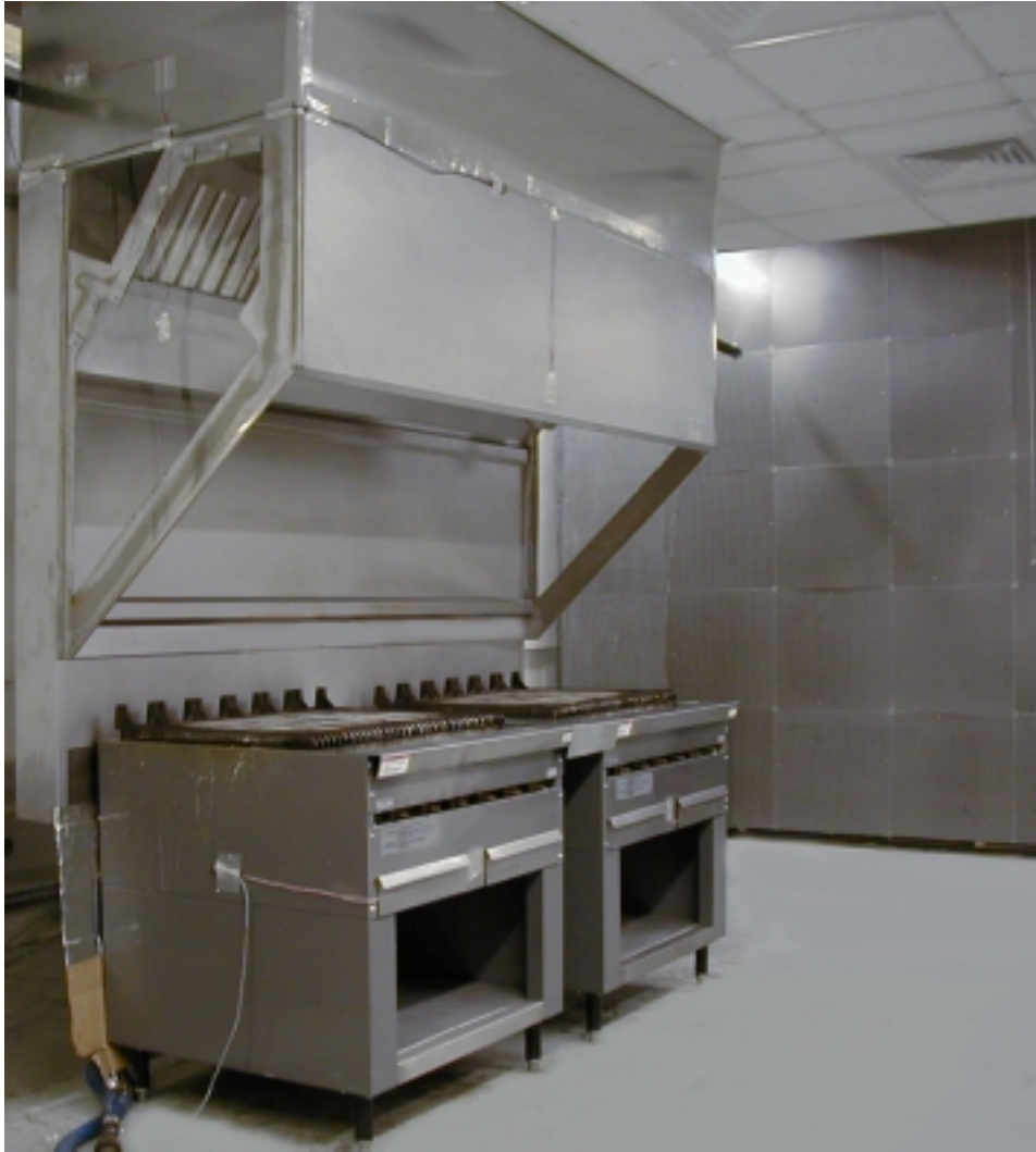
Figure 11: Two Gas Charbroilers under an 86-in Long Proximity (Backshelf) Hood with Transparent Partial Side Panels
