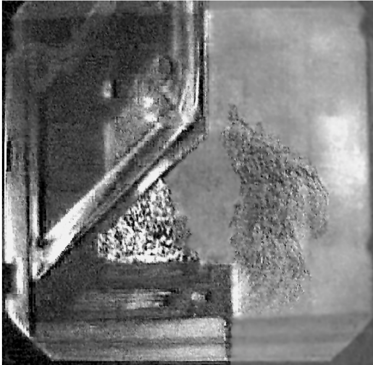
Figure 85: Schlieren Image of C&C with Two Griddles Idling under the Proximity Hood Exhausting 1250 cfm with 325 cfm MUA from the Backwall Supply
