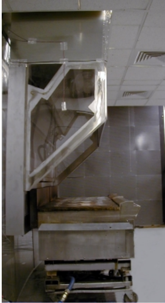
Figure 21: Test Set-Up of the Proximity Hood and Two Gas Griddles as Viewed from the Schlieren Optical Box
