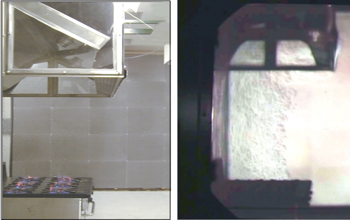
Figure 4: Naked Eye and Schlieren Optical System Views of an Open Range Top with Burners on, under Canopy Hood
