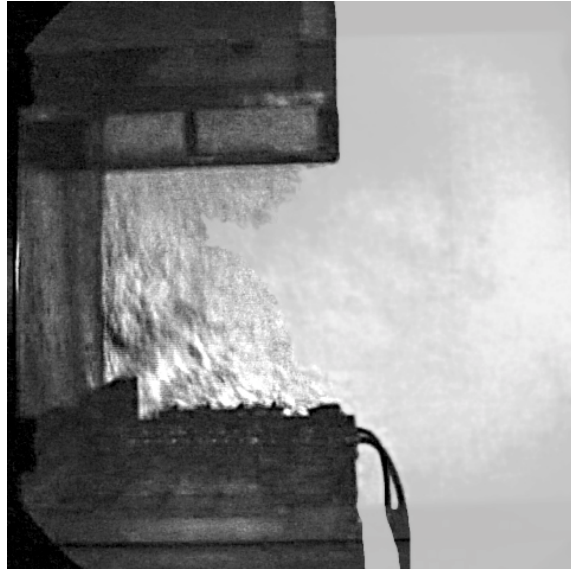
Figure 18: Schlieren View of Exhaust Only Canopy Hood and Two Griddles Simulated Cooking at 2525 CFM Exhaust Flow Rate Showing C&C
