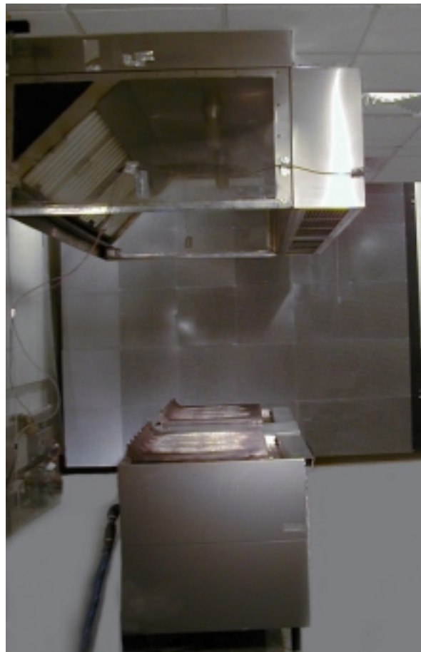
Figure 29: View of Two Charbroilers under a Wall Mounted Air Curtain Canopy Hood from the Perspective of the Schlieren System
