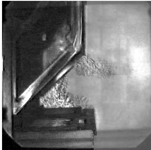
Figure 61: Schlieren View of a Proximity Hood and Two Charbroilers with Simulated Cooking at 1250 CFM Exhaust and 1000 CFM Front Center 4-Way Diffuser Airflow Rates Showing Spillage
