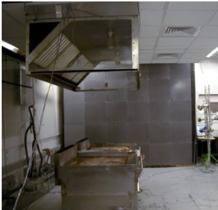
Figure 17: Test Set-Up of the Exhaust Only Canopy Hood and Two Gas Griddles as Viewed from the Schlieren Optical Box
