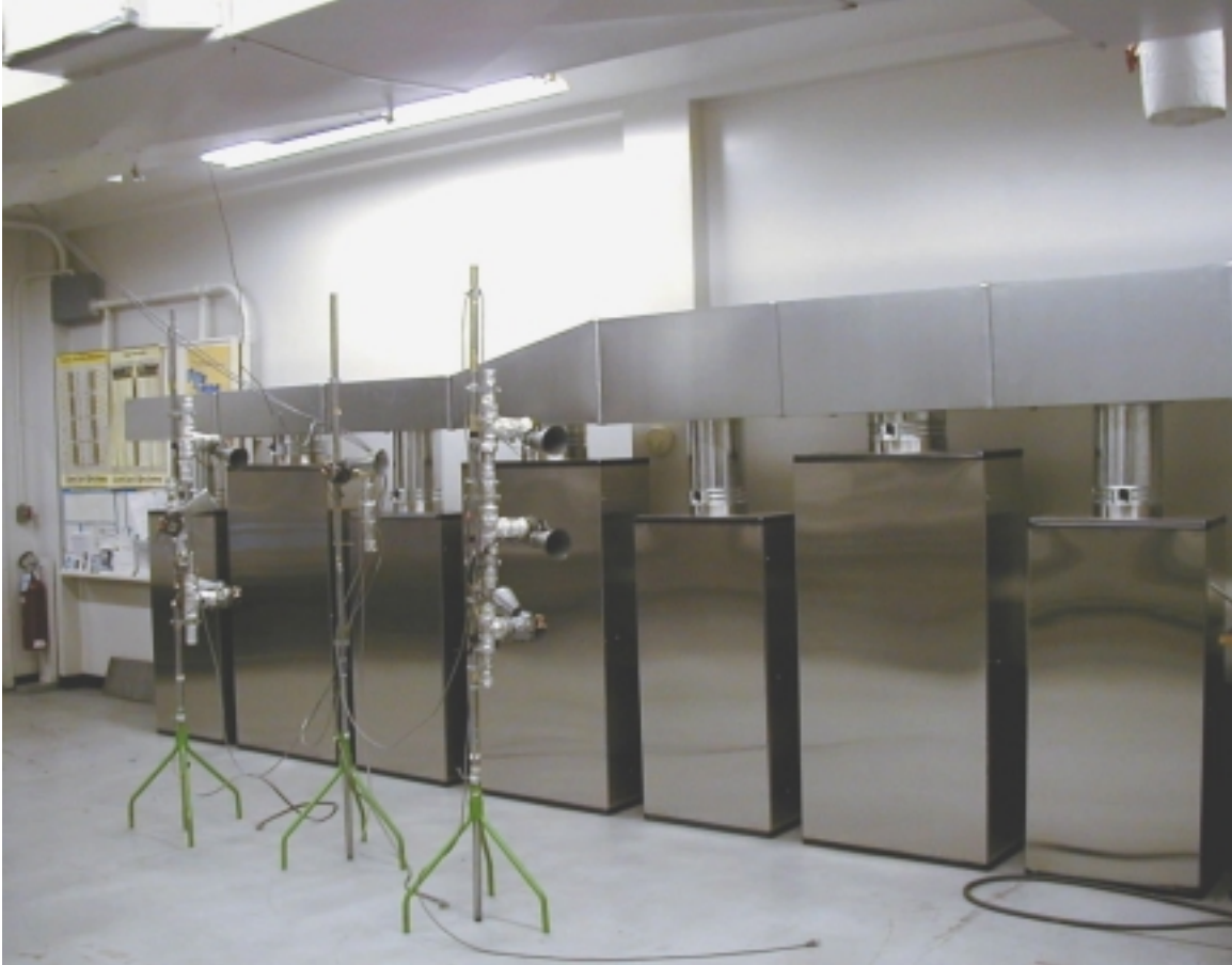
Figure 15: Floor Mounted Displacement Ventilators as Used for the Baseline Replacement Air Case
