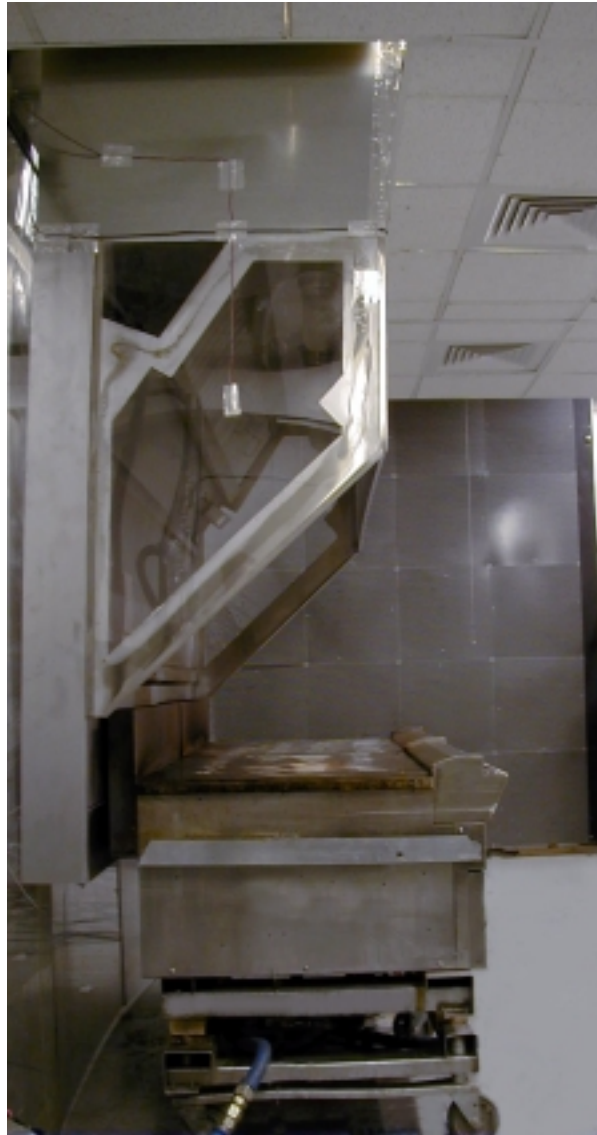
Figure 59: Test Set-Up for Proximity Hood and Two Gas Griddles as Viewed from the Schlieren Optical Box
