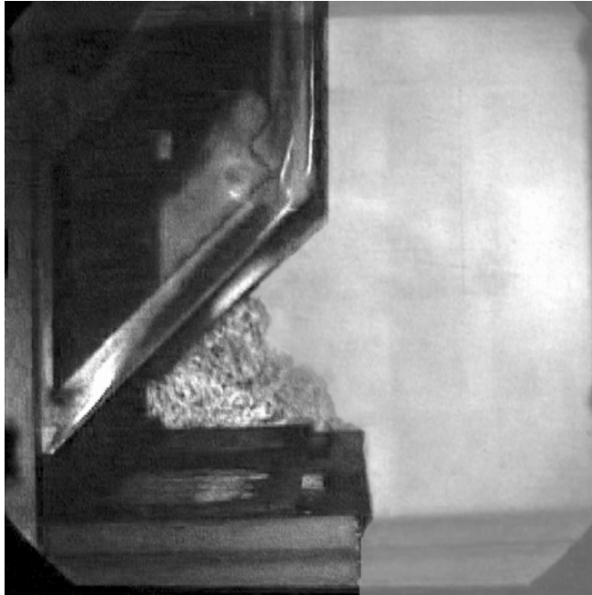
Figure 22: Schlieren View of a Proximity Hood and Two Charbroilers Simulated Cooking at 1250 CFM Exhaust Flow Rate Showing C&C
