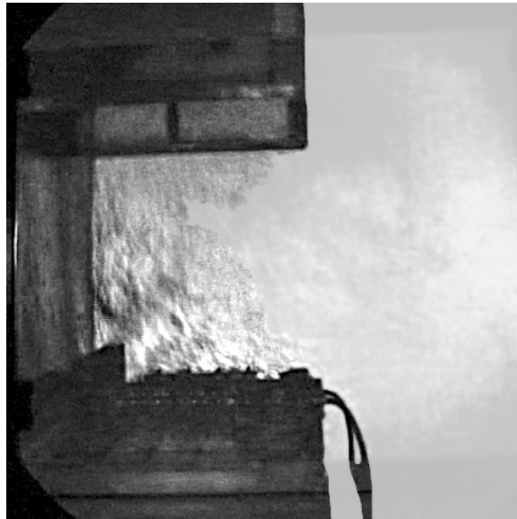
Figure 56: Schlieren View of C&C of Exhaust Only Canopy Hood and Two Griddles Simulated Cooking at 2525 CFM Exhaust and 1000 CFM Front Center 4-Way Diffuser Airflow Rates
