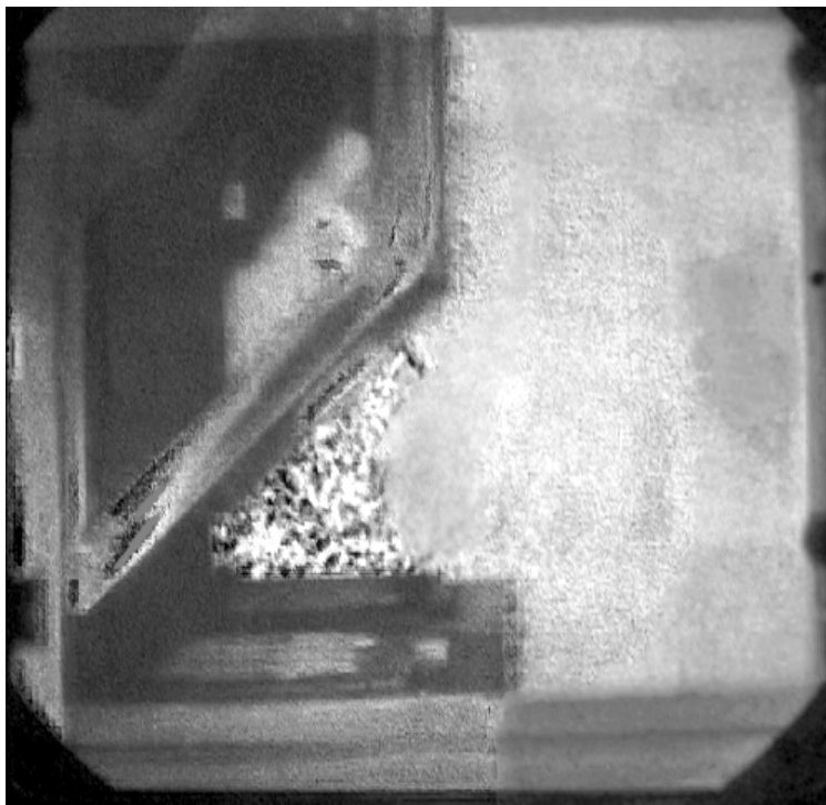
Figure 86: Schlieren Image of Spillage from the Proximity Hood Exhausting 1250 cfm with Two Griddles Idling with 940 cfm MUA from the Backwall Supply
