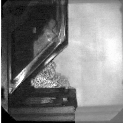
Figure 60: Schlieren View of a Proximity Hood and Two Charbroilers with Simulated Cooking at 1250 CFM Exhaust and 425 CFM Front Center 4-Way Diffuser Airflow Rates Showing C&C
