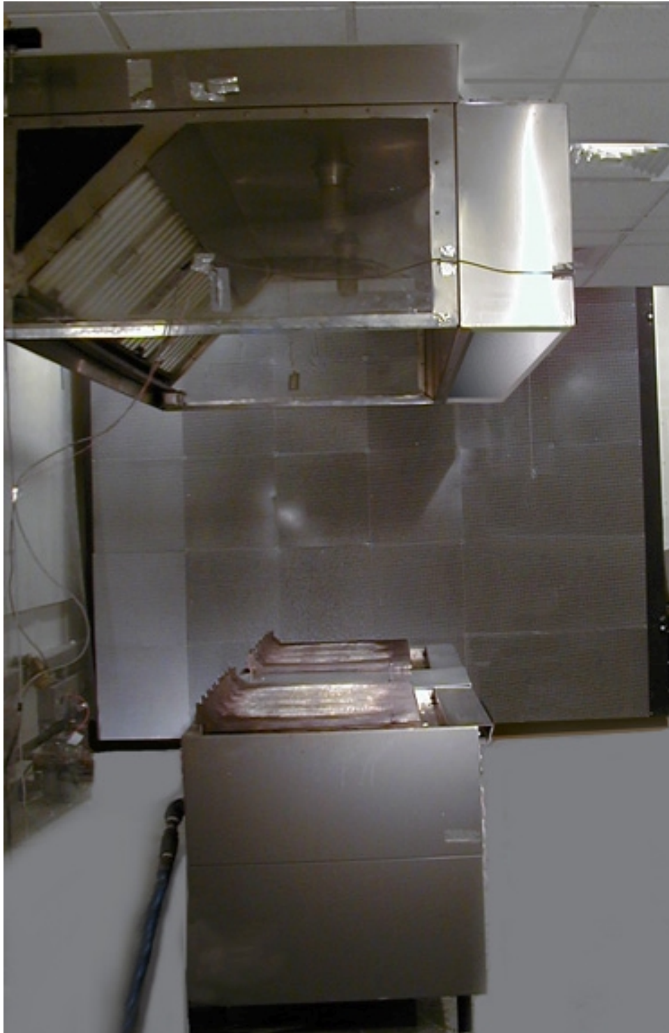
Figure 39: Test Set-Up of the Front Face Supply Hood and Two Gas Charbroilers as Viewed from the Schlieren Optical Box
