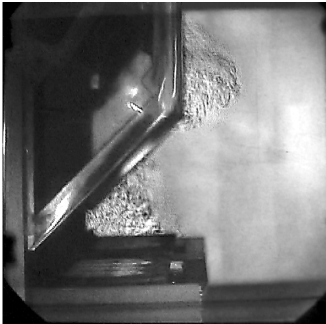
Figure 23: Schlieren View of a Proximity Hood and Two Charbroilers with Simulated Cooking at 1050 CFM Exhaust Flow Rate Showing Spillage
