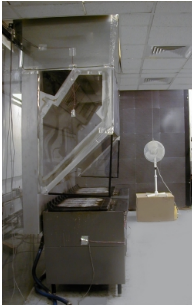
Figure 12: Side View of Two Gas Charbroilers under an 86-in Wide Proximity (Backshelf) Hood with Transparent Partial Side Panels
