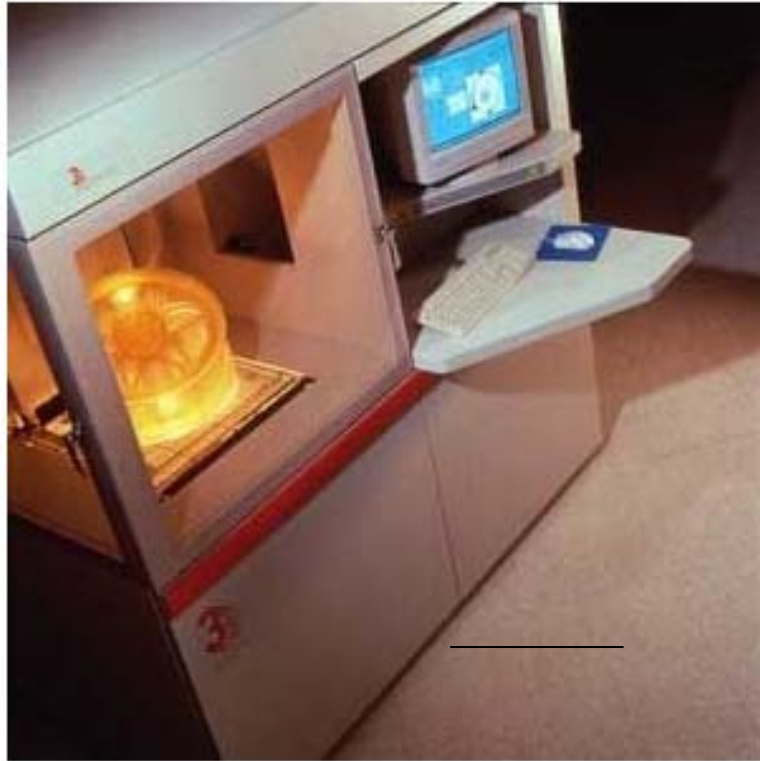
FIGURE 14: Console necessary for rapid prototyping using stereolithography method.
