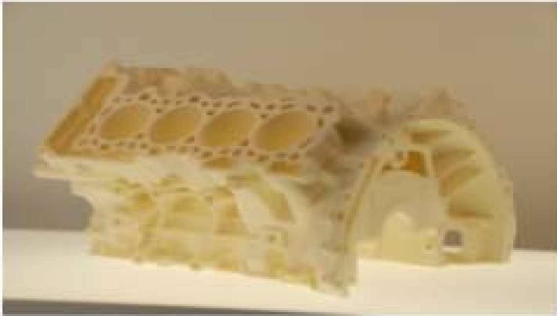
FIGURE 5: Model of engine block produced by Laser Sintering methodology. This part was fabricated using the EOSINT P700 machine with a build volume of 700x380x580 mm. It is one example of a large part that can be produced. Please note the detail. The dimensional tolerances required were met by the process also.
