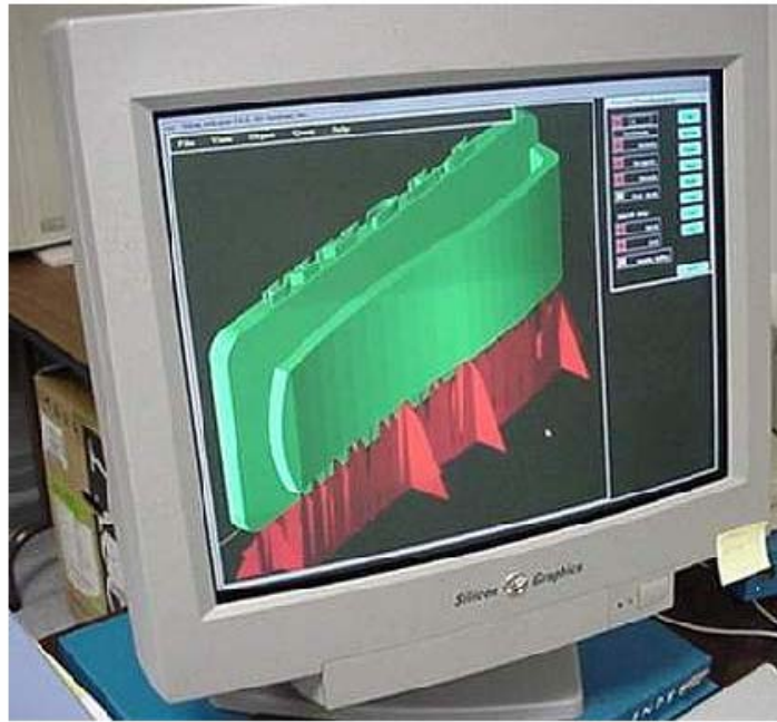
FIGURE 13: CRT showing a 3-D model required prior to prototyping.
