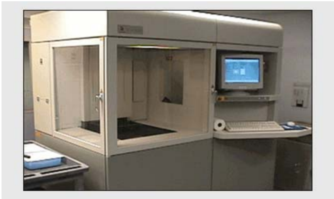
FIGURE 15: A second version of equipment necessary for producing a component by stereolithography.
