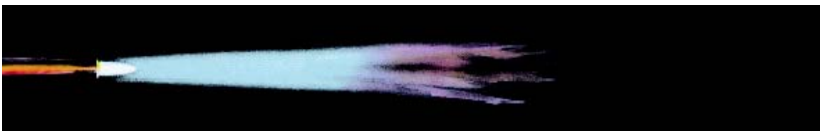
Oxidizing Flame (Acetylene and excess oxygen, 6300°F)
