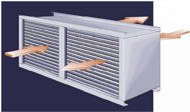
Figure 4 Heat Exchanger for waste heat recovery
