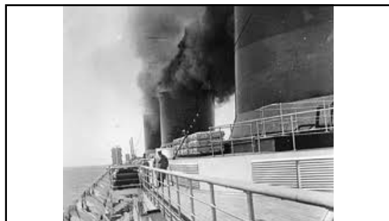
Another problem noticed by passengers on her maiden voyage was soot from the funnels. The forward motion of the ship spread it back across the sun deck, mainly on first-class passengers at play.
