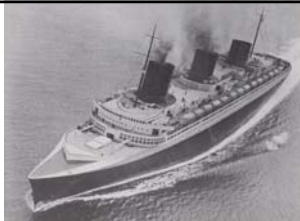
Another important innovation in Yourkevitch's design for the Normandie was the first enclosed Whaleback Bow for an ocean liner. It featured a convex deck housing all equipment/machinery for lowering and/or raising the three, 16-ton bow anchors (there was one, 12-ton anchor at the stern) and a ten-foot high Breakwater (for preventing crashing waves from reaching the superstructure/decks). Made of Teak wood, the curve of the Whaleback's deck served two purposes; decrease wind resistance and disperse quickly the tremendous weight of water crashing over the bow in rough seas. Aesthetically, the Whaleback Bow and concealed deck fittings throughout the superstructure gave Normandie a sleek modern, streamlined appearance. Whaleback Bows and breakwaters are a common feature on modern liners.
