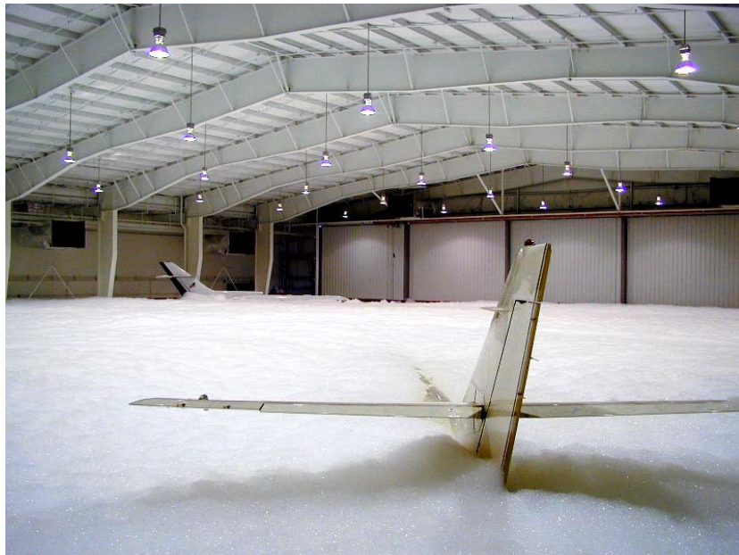
Figure A2.4. Low-Level High-Expansion Foam After 15-Minute Discharge
