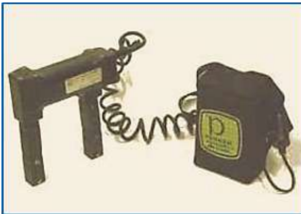
Portable yoke with a battery pack
