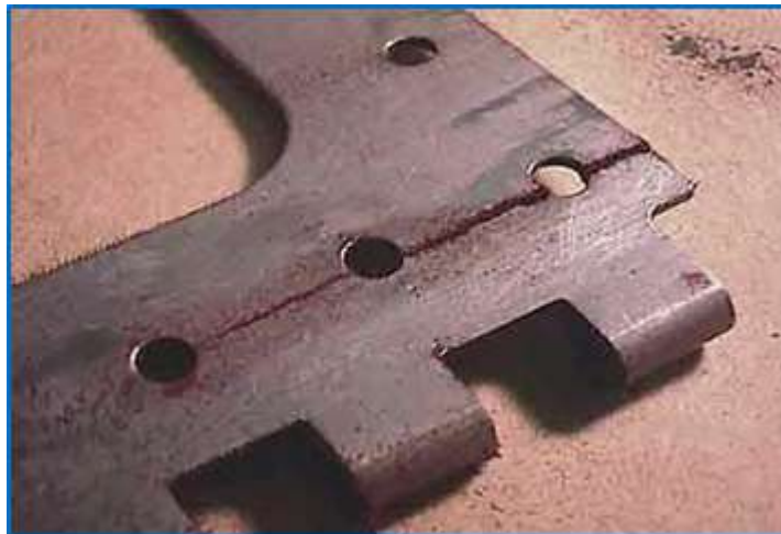
Indication of cracks running between attachment holes in a hinge
