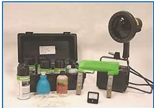
Portable magnetic particle kit
