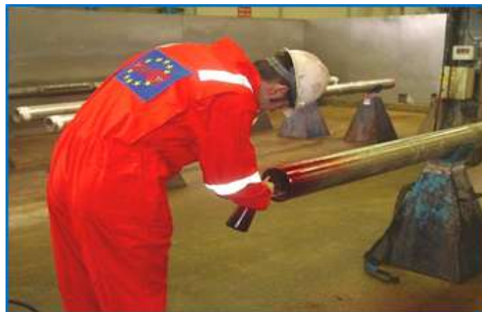
Pipe - LP Inspection
