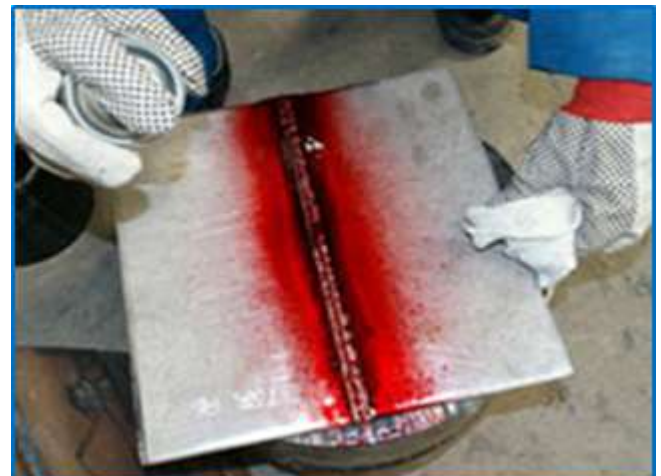
Welding - LP Inspection
