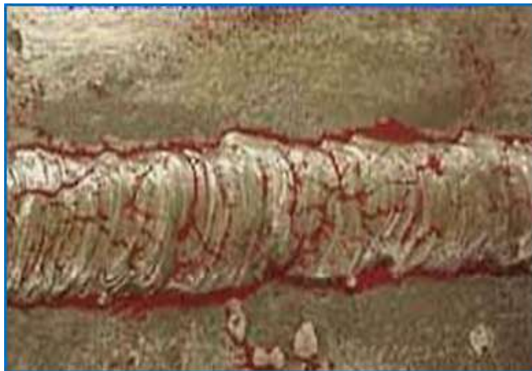
Indication of cracks in a weldment
