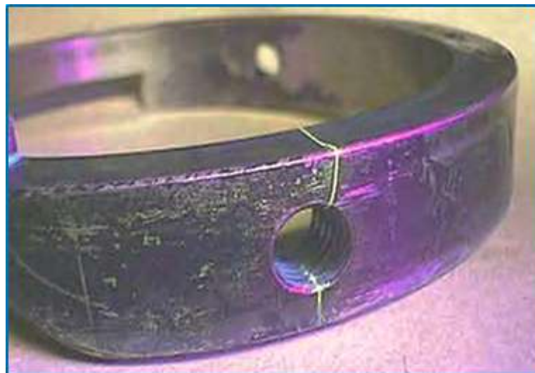
Magnetic particle wet fluorescent indication of cracks at a fastener hole.
