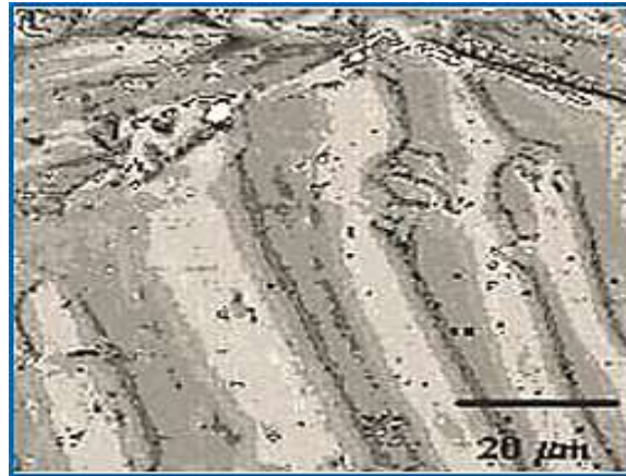
Magnetic Force Microscopy (MFM) image showing the magnetic properties in a piece of heat treated carbon steel.
