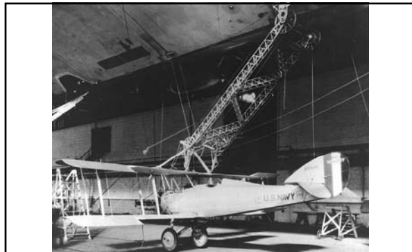
Above: caption: "Vought UO-1 observation airplane attached to the trapeze of USS Los Angeles (ZR-3) during mating experiments in the airship hangar at Naval Air Station Lakehurst, New Jersey, 15 December 1928."
