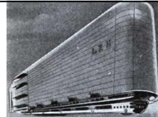
"A gigantic dirigible which would have an all metal body made of corrugated sheet steel, and which would be so durable as to eliminate the need of the customary hangar, is the novel craft recently designed by an eminent Russian inventor, Konstantin Ziolkowski. This craft will expand or contract according to the interior gas pressure."
