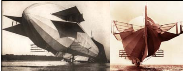
"...The German government became interested and commissioned him to build a larger ship, the ill-fated LZ-4, with 100-horsepower motors..."
