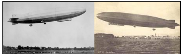
LZ-120's aerodynamically efficient tear-drop shape provided less drag, increased speed and greater lift. It became the basic model from which LZ-126 ( Los Angeles ), LZ-127 ( Graf Zeppelin ), and LZ-129 ( Hindenburg ) were designed and built. LZ-120 carried 706K cubic-feet of hydrogen (later increased to 796,300 during a refit). In the three months after her launch, LZ-120 made 103 flights and carried almost 2,500 passengers, 11K lbs of mail, and 6,600 lbs of cargo. LZ-120 (left) was taken from DELAG by the Military Inter-Allied Commission of Control and delivered to Italy on July 3 rd 1921, where it was renamed Esperia . LZ-121 ( Nordstern ) was built to provide the first international passenger zeppelin service, with plans for scheduled flights between Friedrichshafen , Berlin and Stockholm . She was completed in 1920, but the ship was also taken from DELAG by the Military Inter-Allied Commission and delivered to France on June 13 th 1921 and renamed Mediterranee . 184
