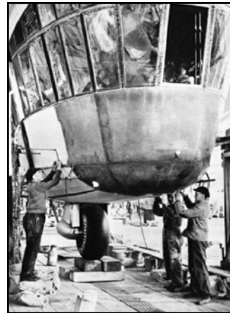
“...The pilot’s cabin of the Hindenburg projects beneath the hull of the airship and is thirty feet long, with a maximum width of eight feet in the centre. The cabin contains the wheelhouse, the map and navigation room, and the direction-finding room...”
