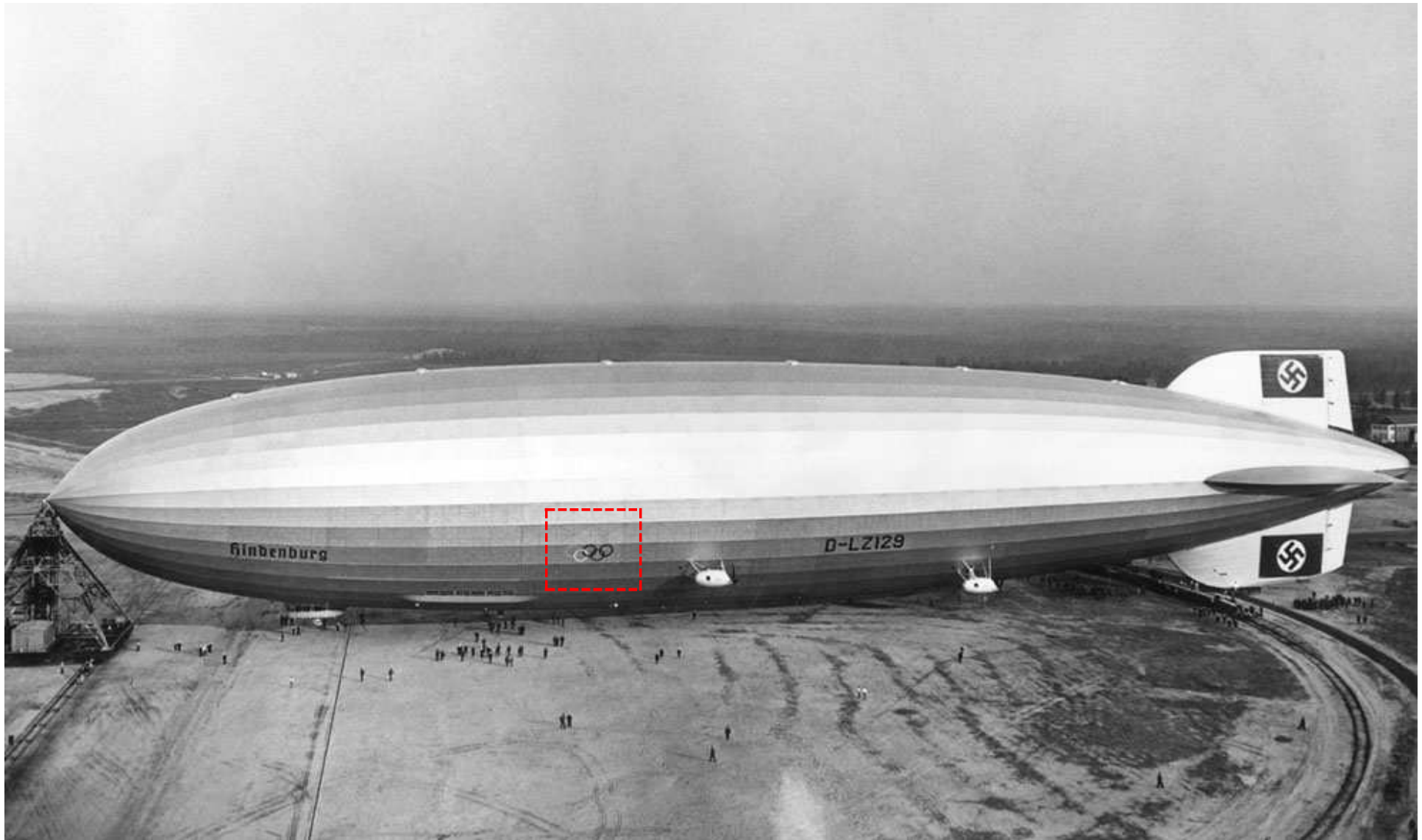
Above: Hindenburg docked at the Lakehurst, NJ Naval Air Station in May 1936. The Olympic rings on the side (highlighted) promoted the 1936 Berlin Summer Olympics (note the circumferential track for the retractable tail-wheel at right).
