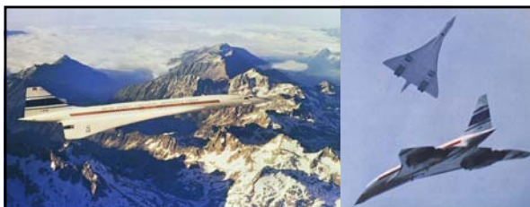
Left: on October 1 st 1969, Concorde 001 - on its 45 th test flight - exceeded Mach 1 for the first time. At an altitude of 36K-feet and seventy-five miles from Toulouse , it held Mach 1.05 for nine minutes. From then on, both Concorde prototypes were to proceed up the Mach scale during flight tests.
