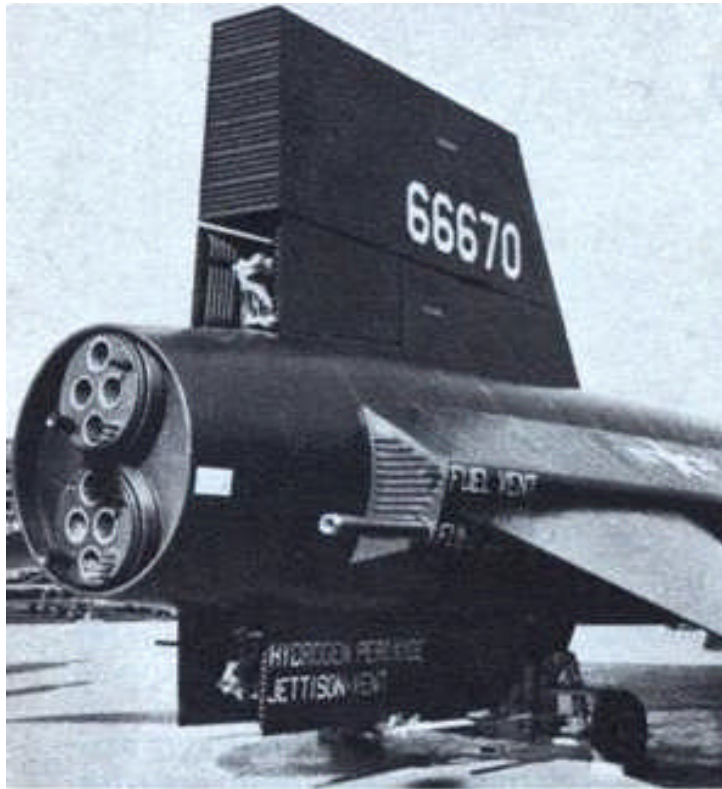
Left: caption: "Left above, exhaust of twin XLR-11 engines. Below, actuator of bottom speed brake."
