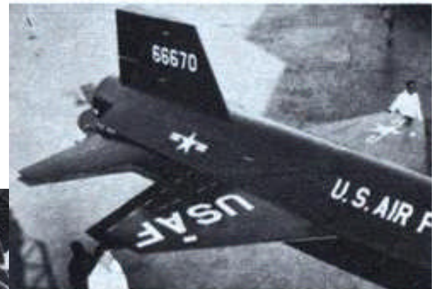
Right: caption: "Nose Contour and trailing edges of wings are surprisingly blunt. In flight, pitch and yaw will be controlled by small ballistic rockets set into nose and wingtips. Bottom part of tail was taken off for rollout. will be replaced for flight. Only movable surfaces on the wings are the flaps."
