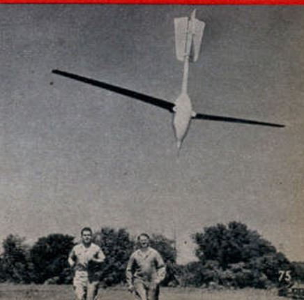
The roto-chute, invented by G.E.'s I. B. Benson, left, lands rocket instruments at easy 27 mph.
