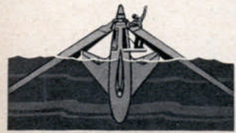
LANDING AT SEA, THE CAPSULE FLOATS UPRIGHT LIKE A BUOY, STEADIED BY ITS FINS AND ROTOR VANES. FOOD, WATER AND SURVIVAL GEAR KEEP PILOT ALIVE UNTIL RADIO AND POSITION LIGHT BRING RESCUERS.
