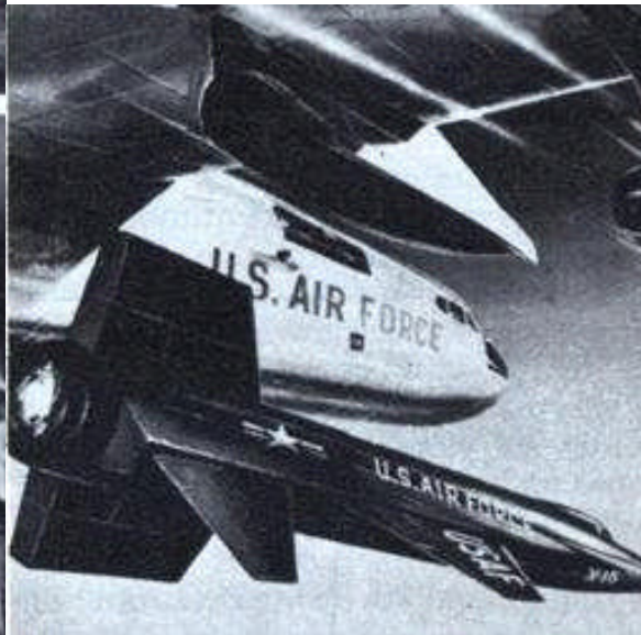
Above: caption: "Drop launching is shown in drawing below. After release from B-52, the X-15 will rocket upward to 100-mile altitude." 158
